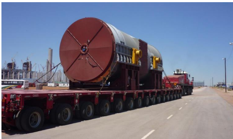
Figure 5: Heavy haulage truck with 16-axle hydraulic trailer transporting a 360 ton generator (source: ALE)
