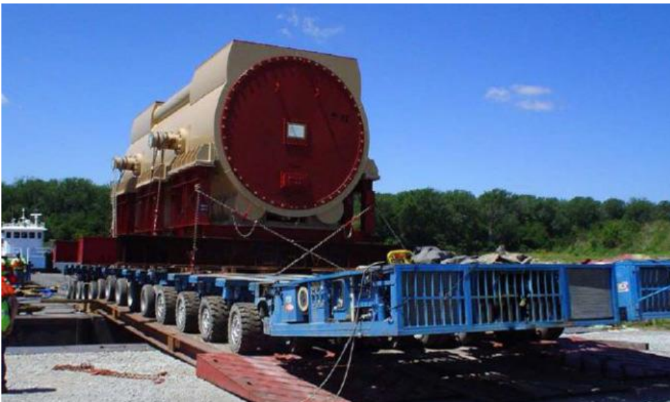
Figure 4: Example of large equipment being offloaded from a barge. Note the levels of the ramp, the barge and the jetty (source: SUBTECH)
