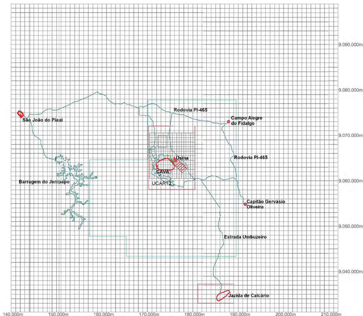
Figure 5.1-17 – Location of receiving points considered for the air pollutants dispersion modelling study.
