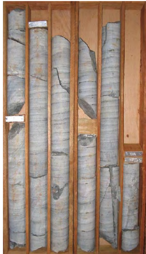
Photo 5.1-2 – Drill core from the Brejo Seco area, of light gray rock, solid, subphaneritic, with inclined incipient foliation and possible silica and carbonate veinlets (mm).
