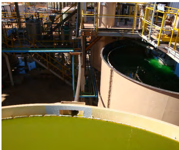
Photo 2.3-9 – Precipitation tanks separating Nickel and Cobalt from unwanted metals from the ore (Fe, Al), by adding limestone.
