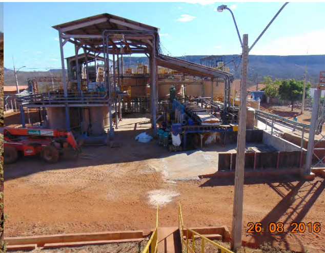
Photo 2.3-8 – Hydrometallurgical Testing Plant that receives the metal-rich solution (PLS) for separation, precipitation, and filtration of the MHP product and the IFC residue (both in solid state).
