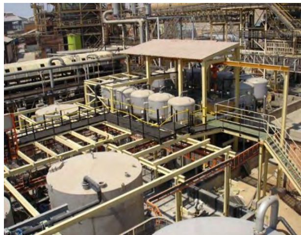
Photo 2.9-8 – Example of a working nickel-cobalt separation (IX) plant, Zambia.
