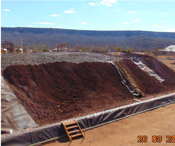
Photo 2.3-7 – View of the plastic pipe network mounted on top of the heaps for slow dripping of them with acid solution diluted with water.
