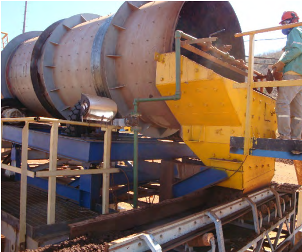
Photo 2.3-3 – Ore agglomeration (fine particles) with application of water + sulfuric acid.
