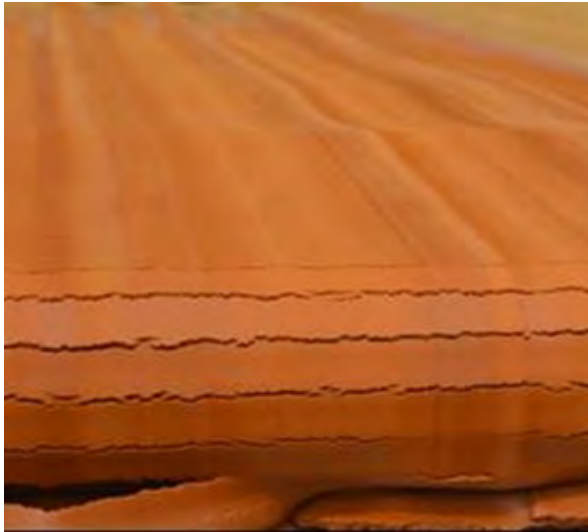
Photo 2.3-13 – Detail of the IFC residue produced also in solid state at the end of the filtration process.
