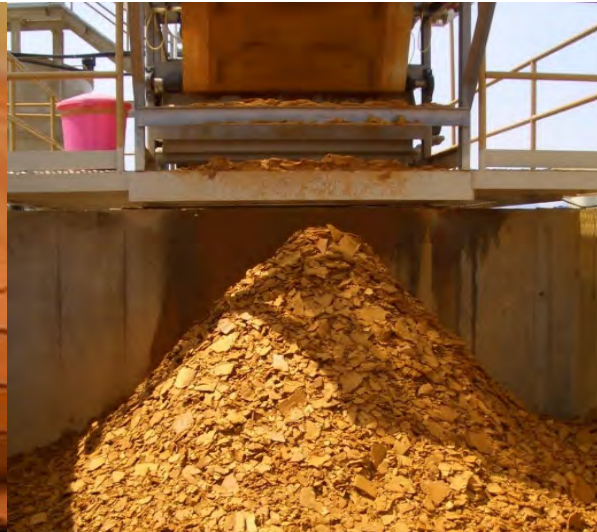
Photo 2.3-14 – Another view of IFC residue produced in solid state after the filtration process.
