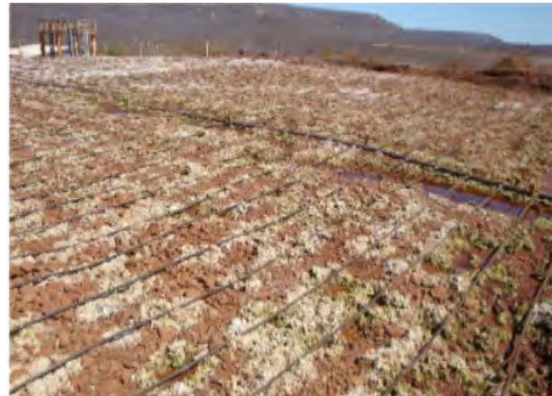
Photo 2.9-2 – Dripping of sulfuric acid solution onto the heaps (Demo Plant)
