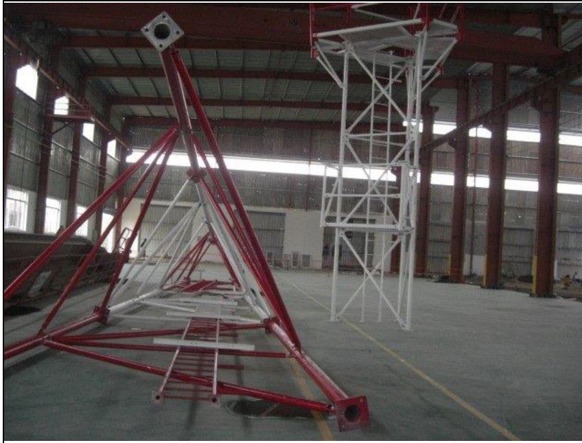
Photo 1: Prefabrication Tower Segements at Steel Factory
