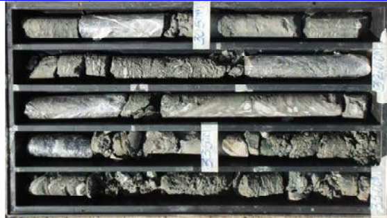
Figure 5-26: Mylonites and recrystalization present in BH-18
