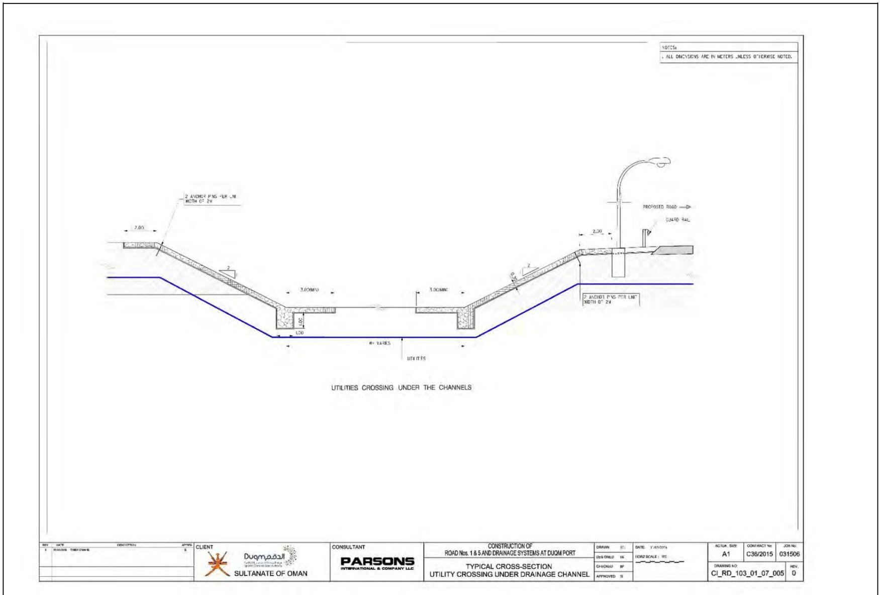
Figure 3-23: Cross-Section of Utilities crossing under the channels.
