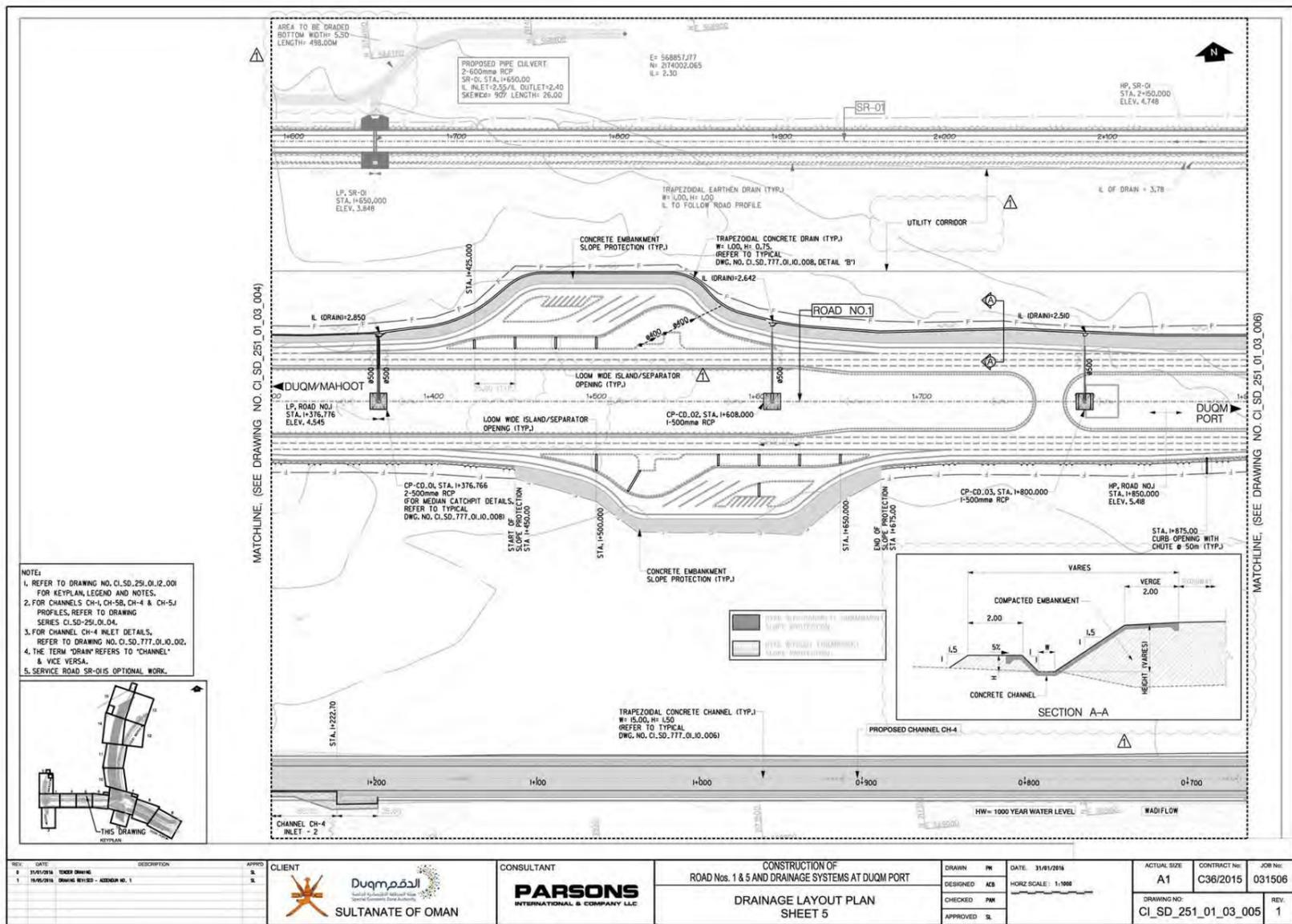
Figure 3-15: Detailed Drainage Layout Plan Section 4 & 5
