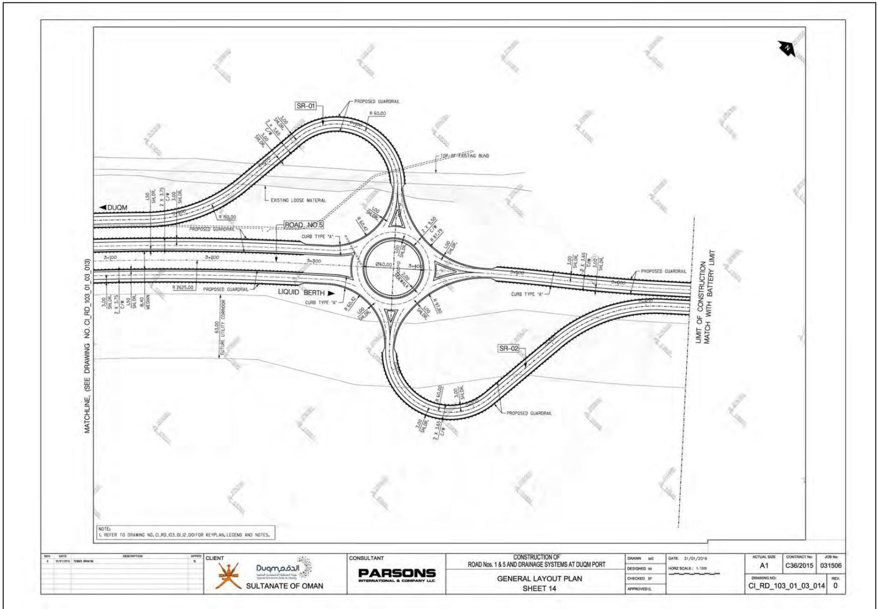
Figure 3-8: Detailed Layout plan of section 14
