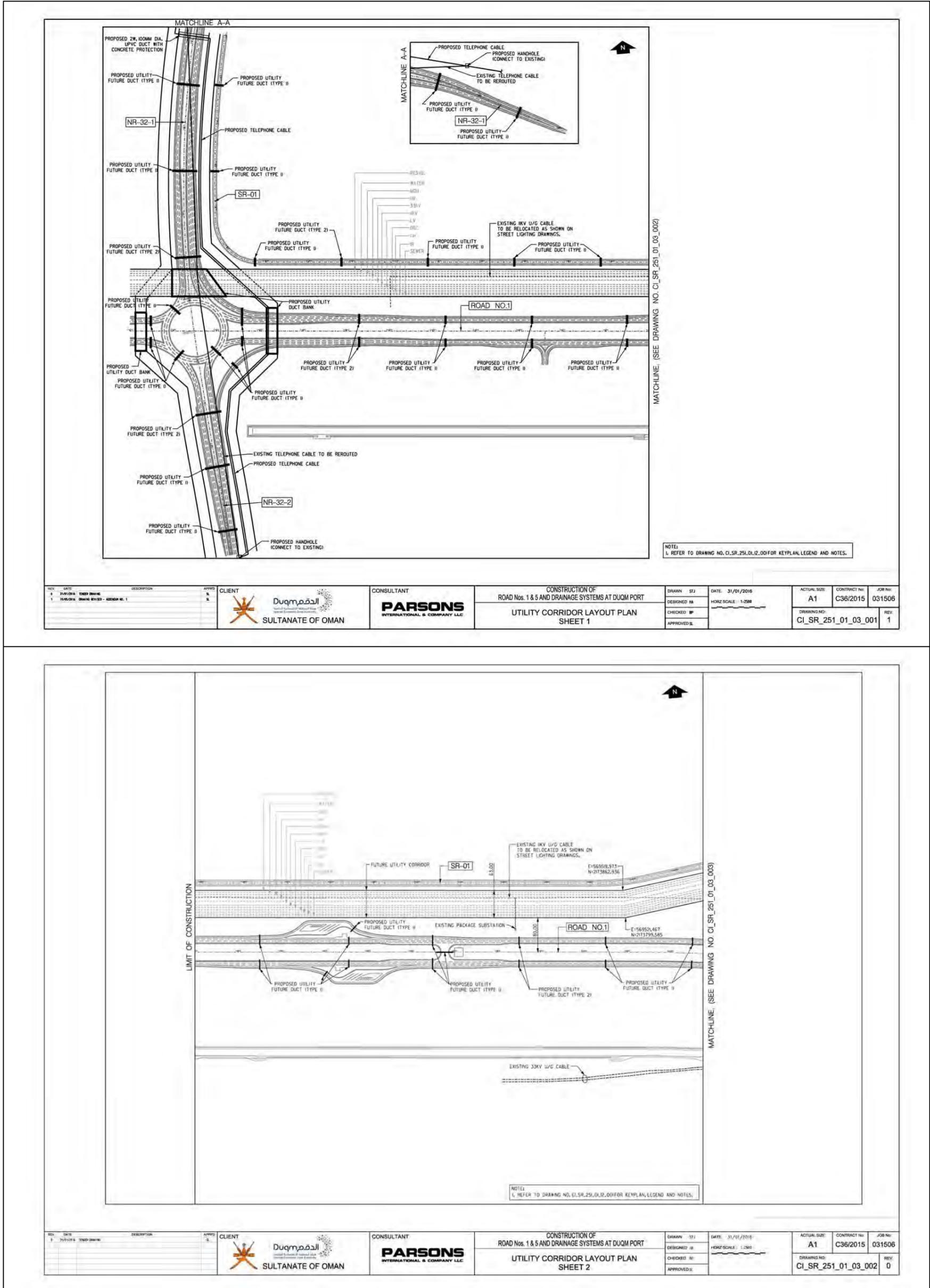
Figure 3-10: Detailed Utility corridor Layout Plan- section 1&2
