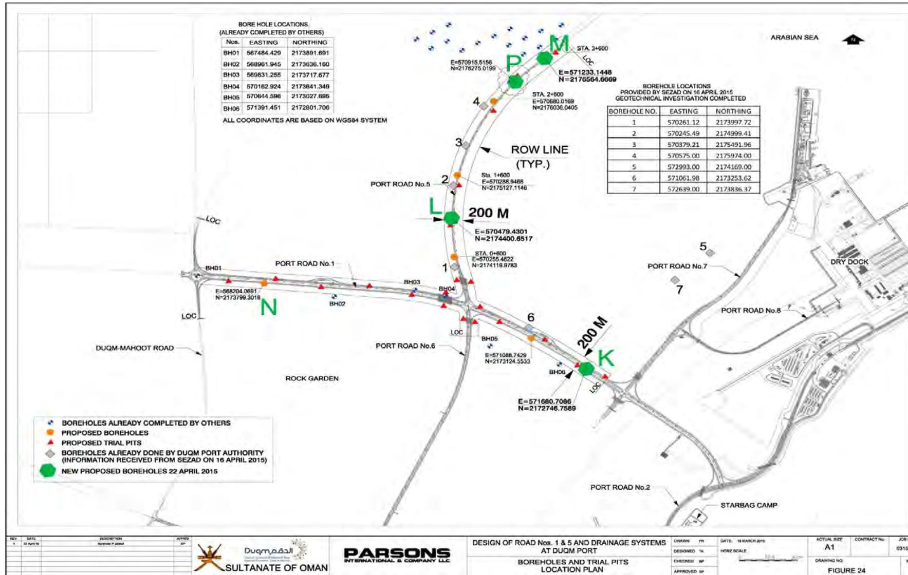
Figure 4-3: Boreholes and Trial Pits Locations
