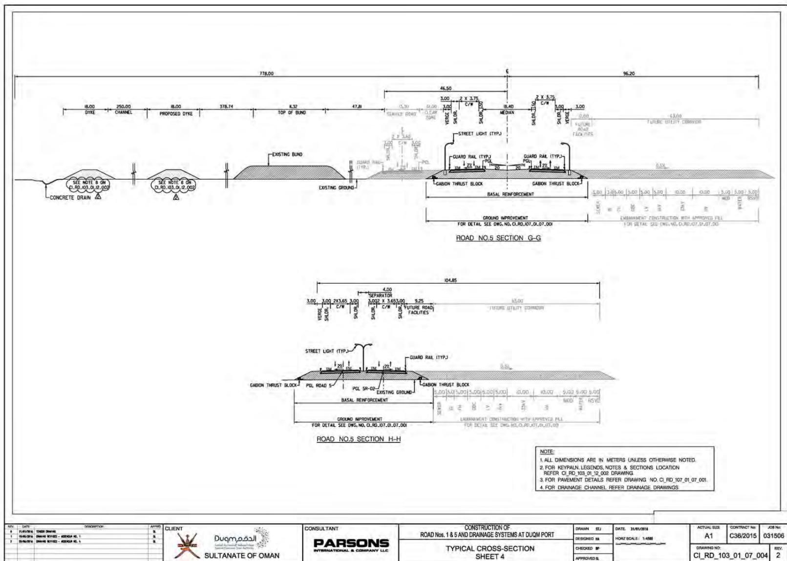
Figure 3-22: Cross-Section Details of Road 5.
