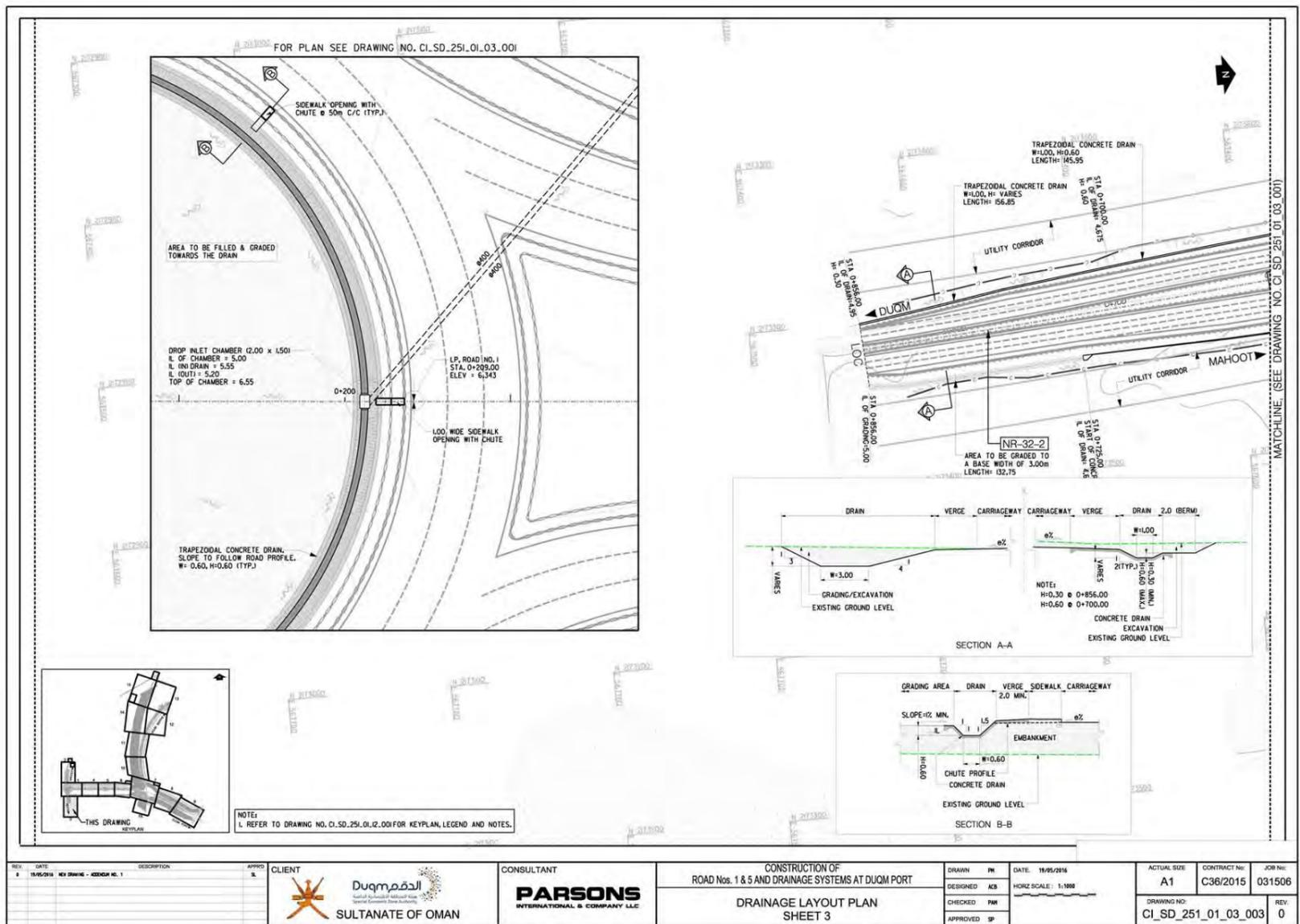
Figure 3-14: Detailed Drainage Layout Plan Section 2 & 3
