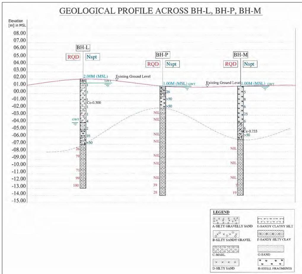
Figure 4-1: Geological profiles across the boreholes
