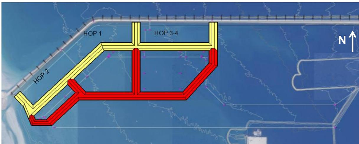
Figure 2-1: Preliminary design for the construction of permanent reclamation bunds (yellow) and temporary bunds (red) [B.3]
