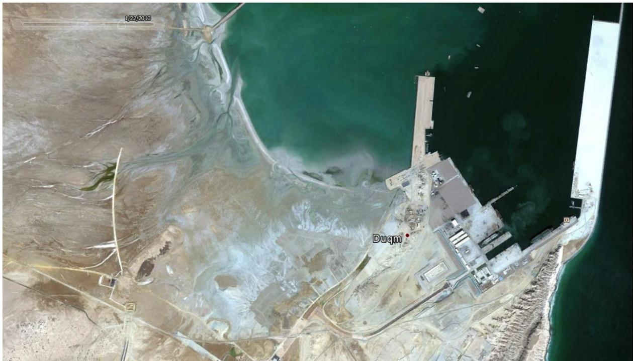
Figure 4-3: Google Earth satellite image dated 22 January 2013, showing construction of temporary Road n. 5 through the wadi area, and filling of the wadi area in the southwest of the Port Future Basin.
