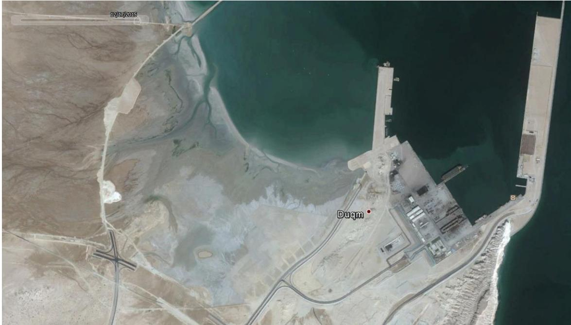
Figure 4-4: Google Earth satellite image dated 17 December 2015, showing filling of the wadi along temporary Road n. 5, and continued filling of the wadi in the southwest of the Port Future Basin
