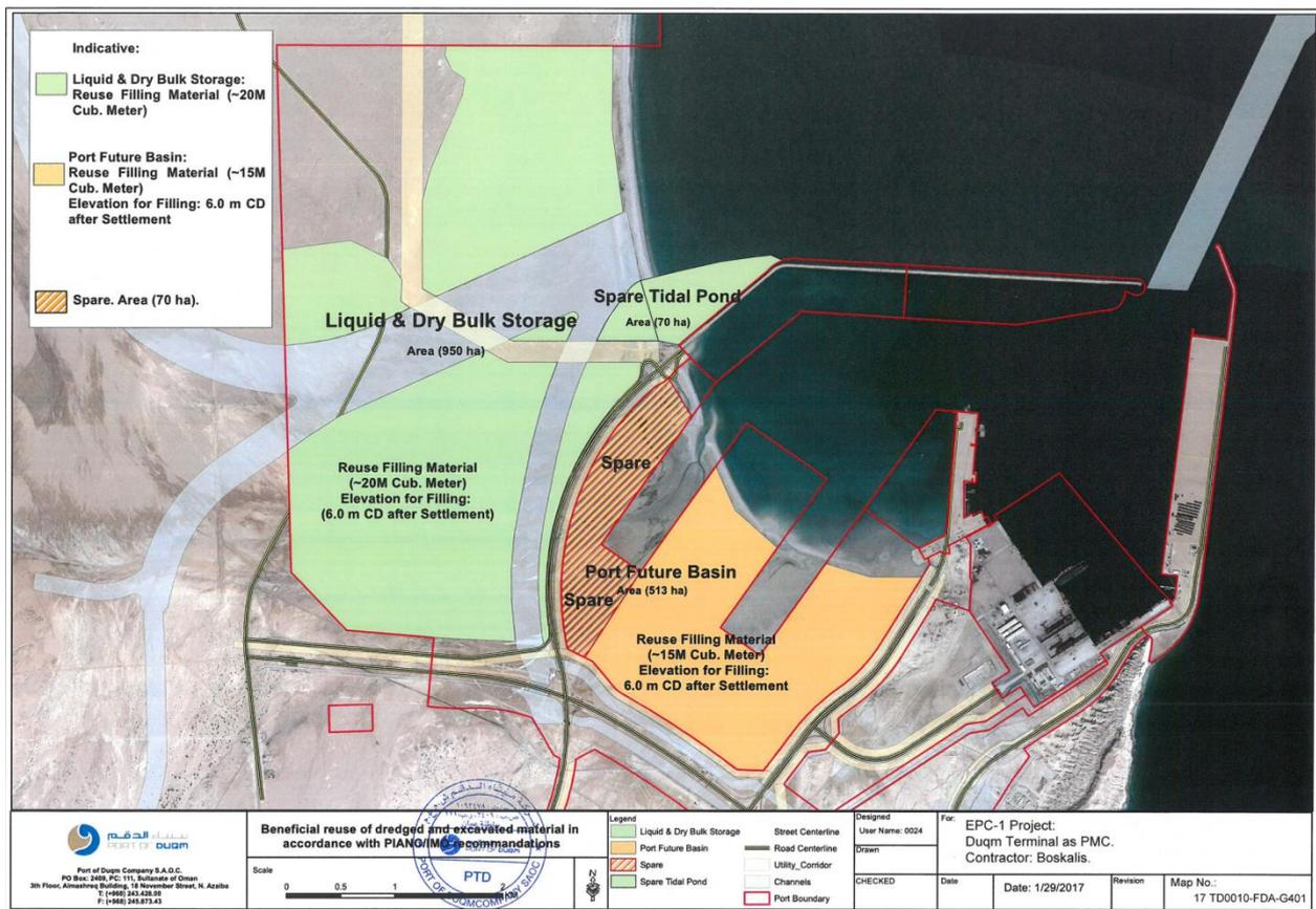
Figure 3-2: Areas identified by Port of Duqm for placement of filling material (revision of 29/01/2017).
