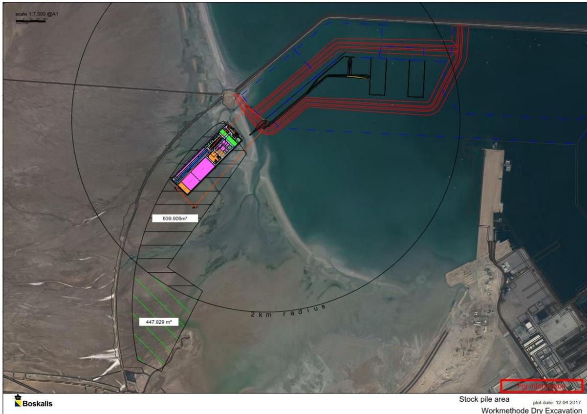
Figure 3-3: Area designated for disposal of dry excavated material (black hatched area, green hatched area to be discussed)
