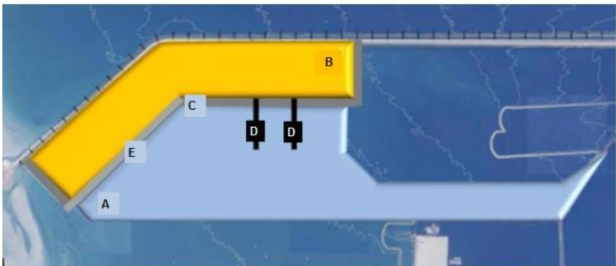
**Figure 1-3: Schematization of the Works (A dredging, B reclamation, C revetment, D jetties and E quaywall)**
