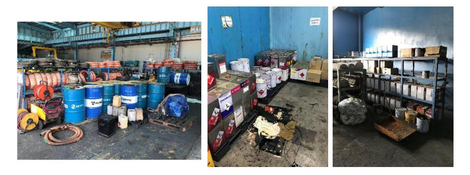
In other areas, batch storage is present, none secondary contained. Left is the maintenance shop, middle is piping pre-treatment (including spill), right is piping paint shop. Risk of contamination is present due to the absence of secondary containment, although the flooring is fully concreted and no stains were observed to move to the outdoor areas. Anticipating the before-mentioned aspects, the risk is classified as **medium**.
