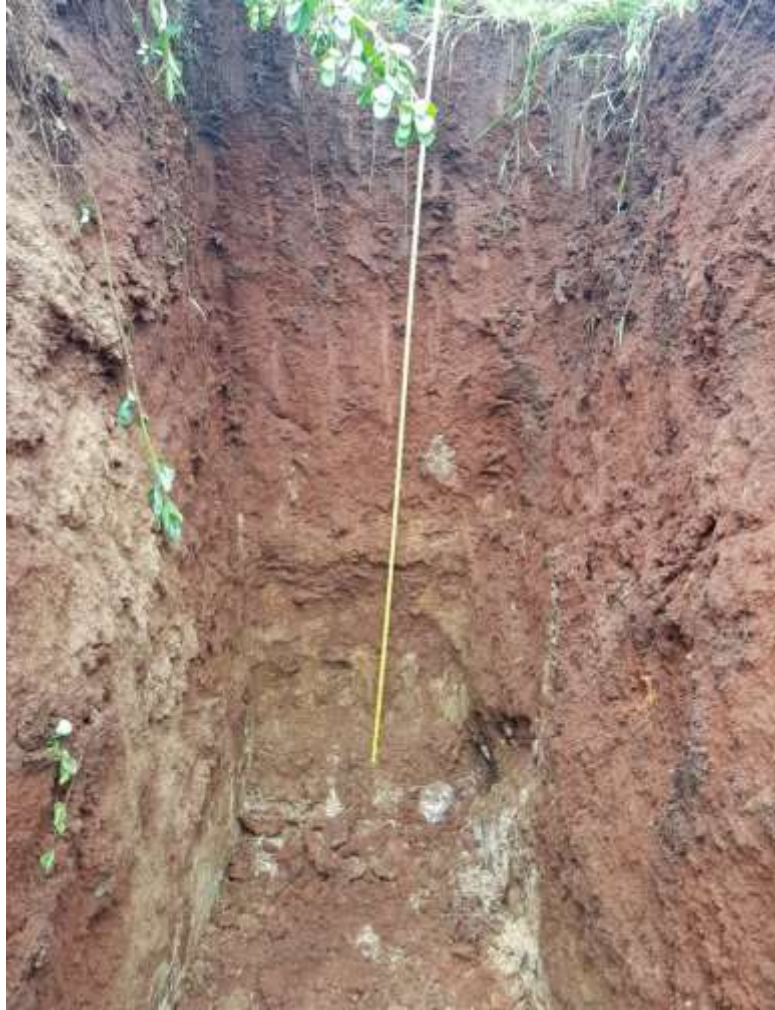
Figure 5.10 Test Pit Profile in Zone Three (Source Aurecon, 2018)
