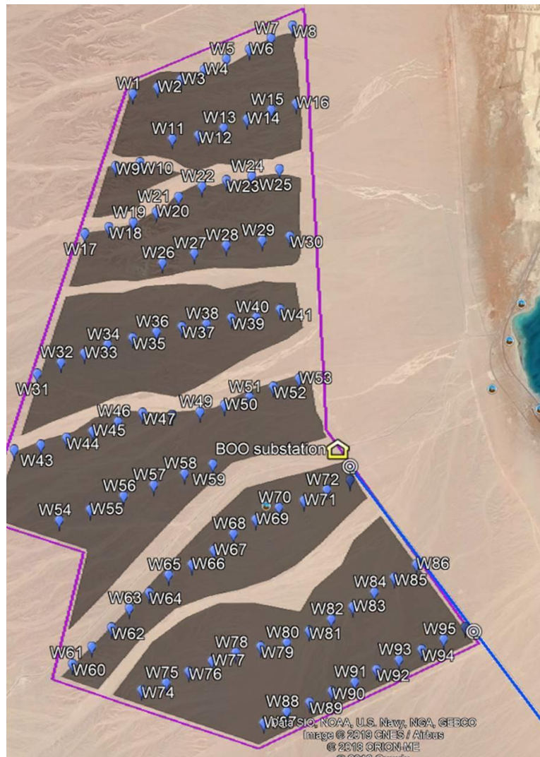
Figure (5): Lekela project layout (96 x 2.6MW)
