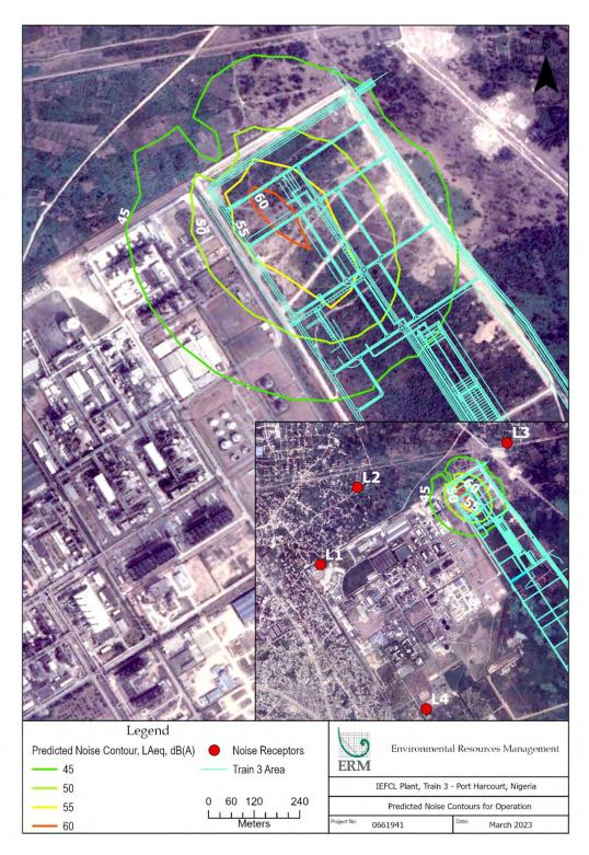
Figure 8-10 Predicted Noise Contours during the Operational Phase
