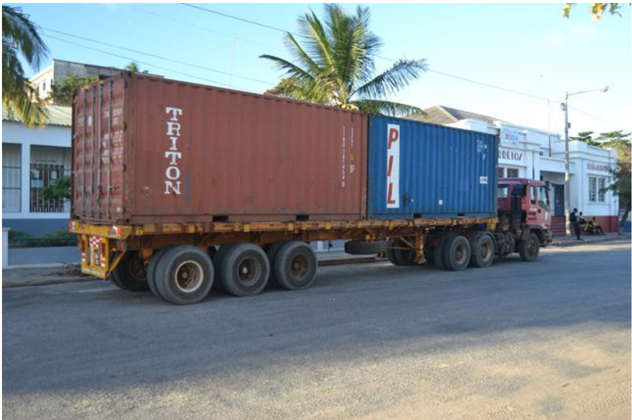
Plate 5.2: A 6-axle articulated truck, carrying two containers each capable of storing 28 tons of goods, delivering to the Port of Pemba on 28 July 2013.
