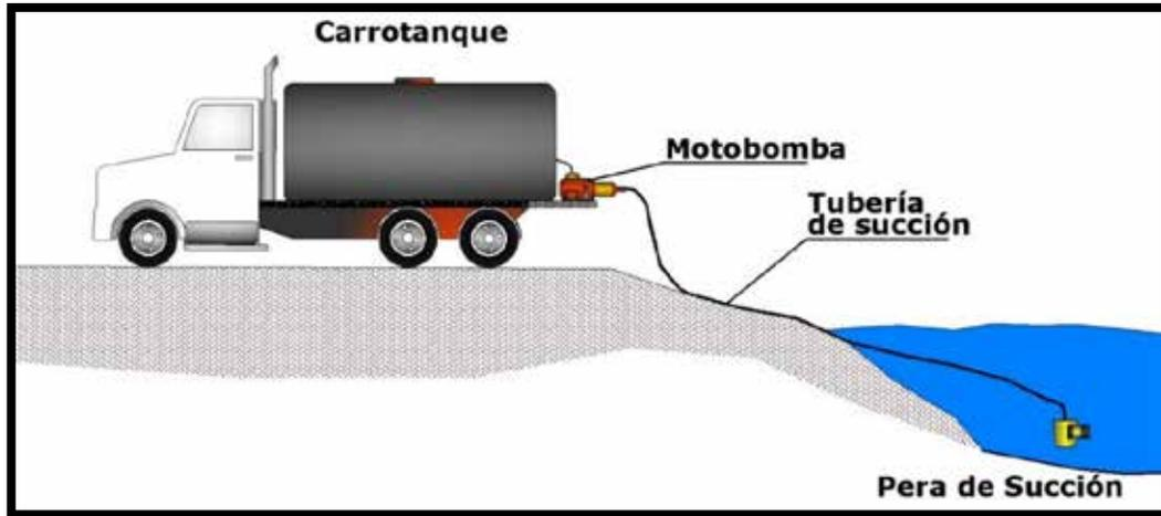
**Figure 7.2 Direct uptake system from tank truck**
