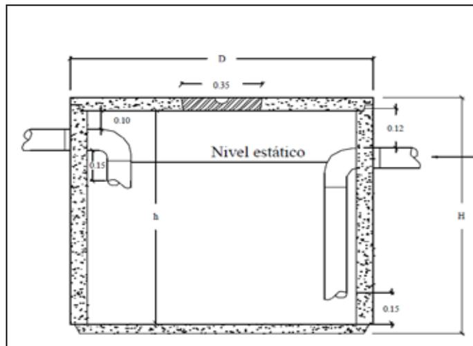
**Figure 7.10: Typical grease trap design**
