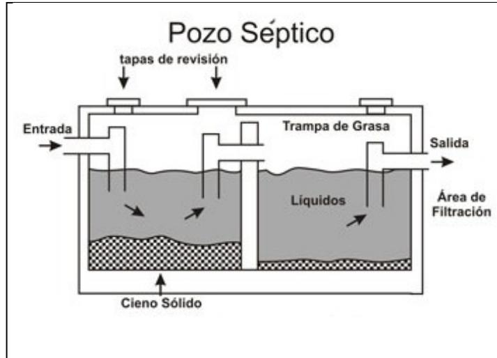
**Figure 7.11: Basic treatment operation**
