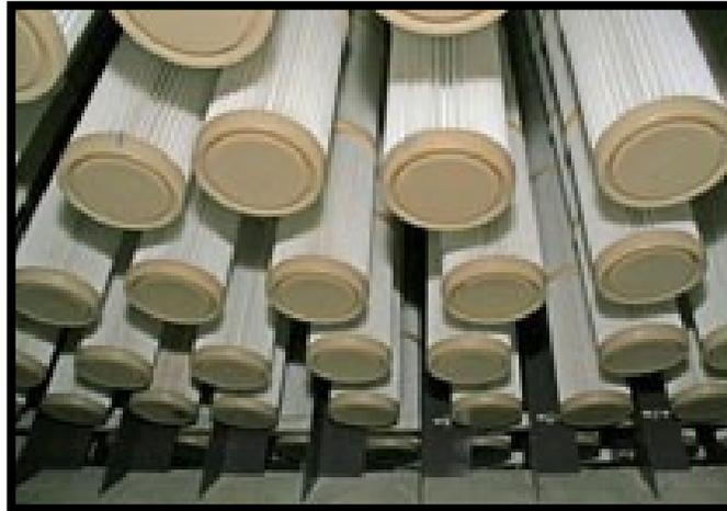
**Figure 7.587: Folding sleeves filter**
