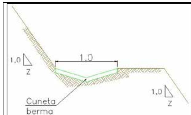
**Figure 7.42 Cut berm ditch**
