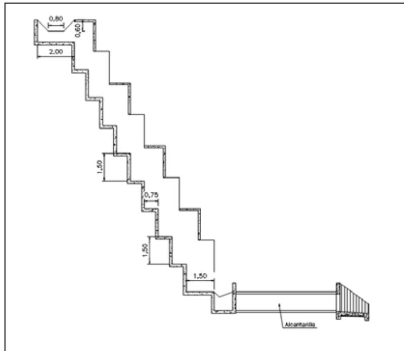
**Figure 7.50 Dissipation structure with inlet box culvert**
