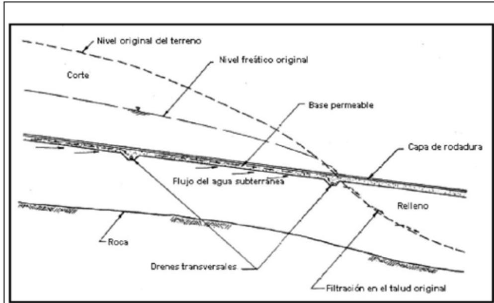
**Figure 7.42 Transvers drain on road in cut with perpendicular alignment to existing contour (profile)**
