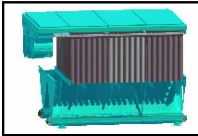
**Figure 7.576: Smooth filter sleeves**
