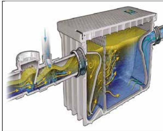
**Figure 7.11: Grease trap operation**
