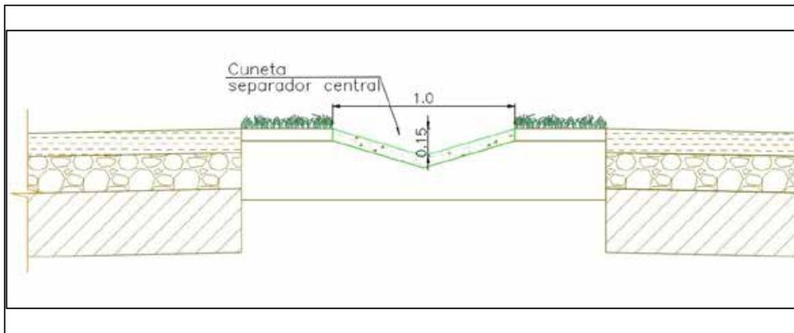
**Figure 7.41 Central separator ditch**
