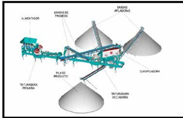
**Figure 7.54 Crushing Plant Model**
