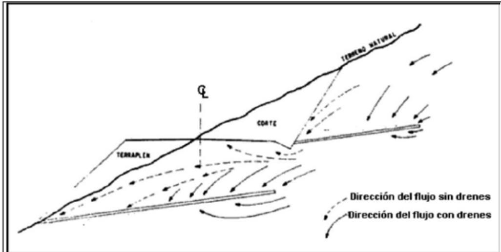
**Figure 7.38 Horizontal drain in hillside cut**
