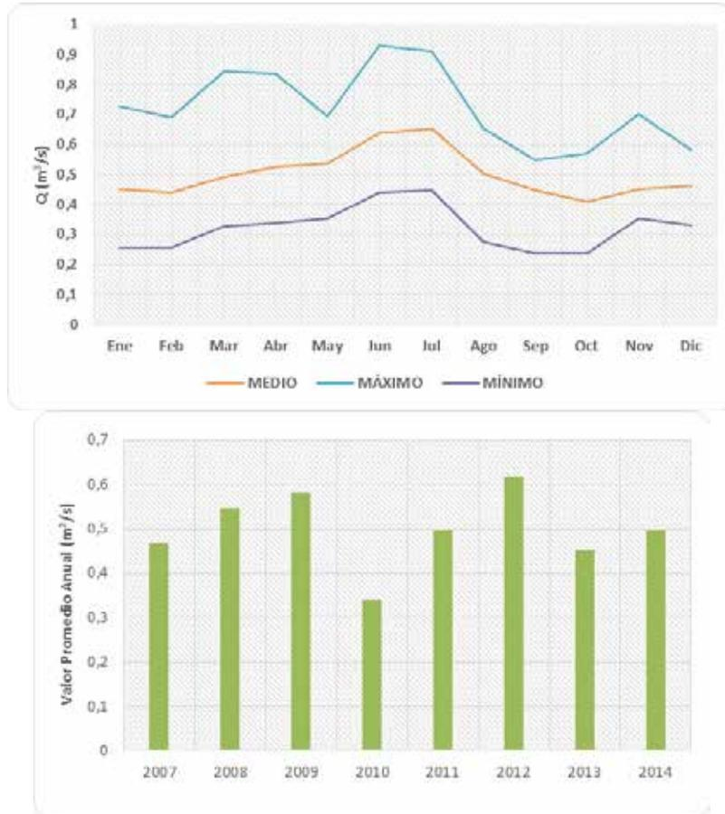
**Figure 7.15 Minimum flow distribution - Casanare Automatic Station(Bobo River)**
