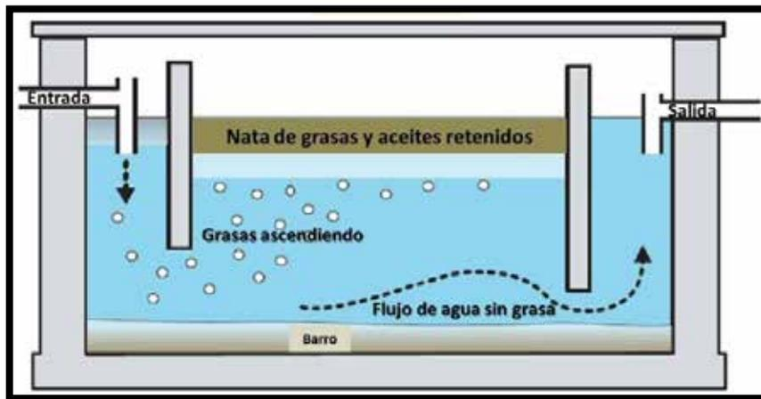
**Figure 7.15 Grease trap operation**
