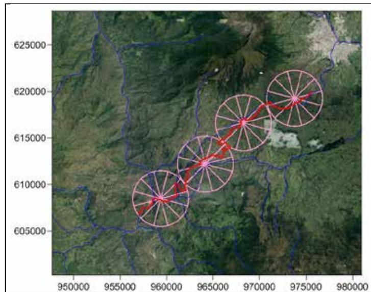
**Figure 7.70** Compartmentalizing the road to determine surface parameters.
