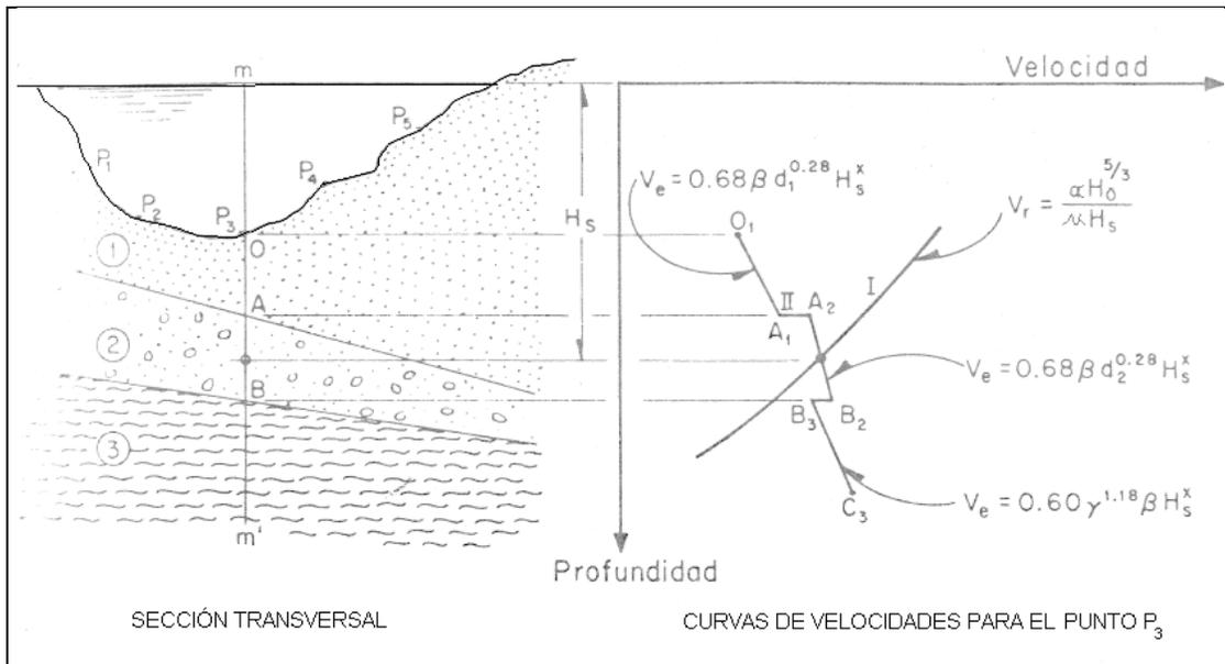
**Figure 7.35 Subsidence calculation by the graphic method**
