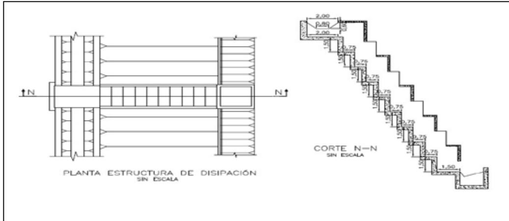
**Figure 7.45 Dissipation structure delivering to ditch**
