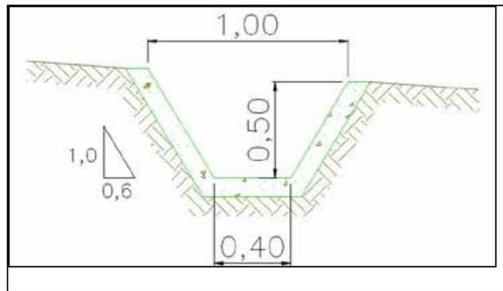
**Figure 7.43 Crown ditches**
