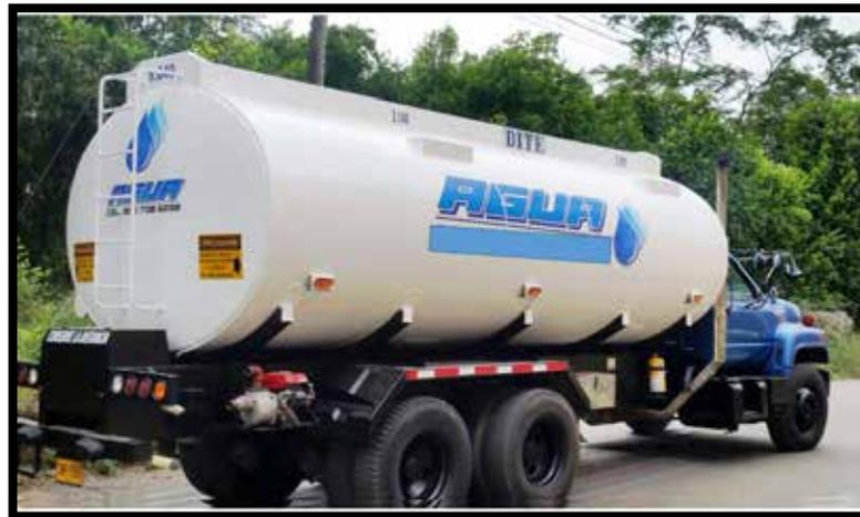
**Figure 7.3 Tank truck for water transport**
