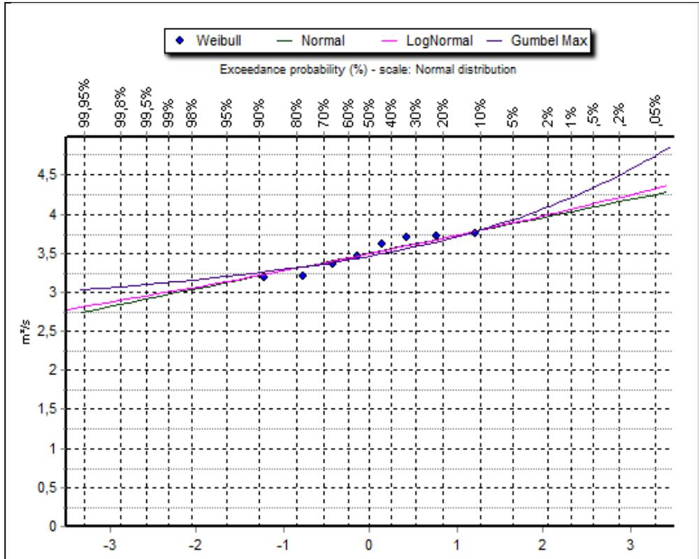
Figure 7.4 Minimum Flow frequencies - Casanare Automatic station
