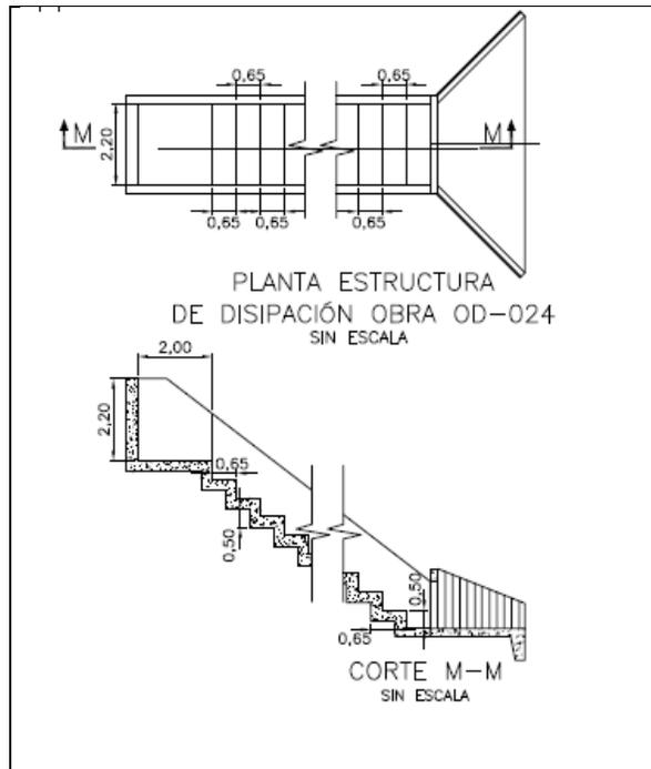
**Figure 7.46 Dissipation structure to outlet**
