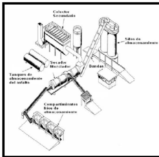
**Figure 7.554: Asphalt plant continuous production scheme**
