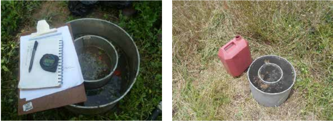
Photograph 7.22 Descent of the Sheet of Water in the Infiltration Test
