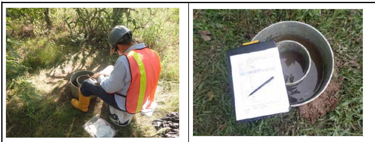
Photograph 7.23 Recordings of Infiltration Tests – Point One (1).
