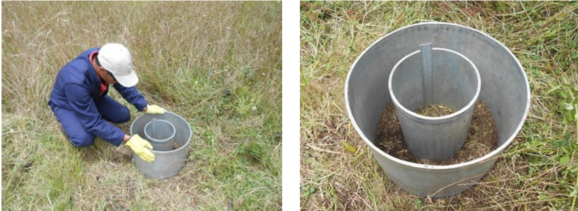
Photograph 7.20 Installation of Infiltrometer Before Infiltration Test
