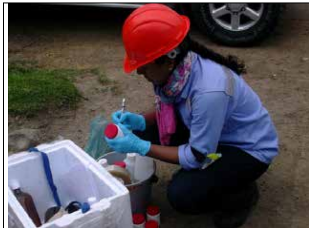
Photography 5.159 Collection of water quality analysis samples, downstream La Marquesa creek
