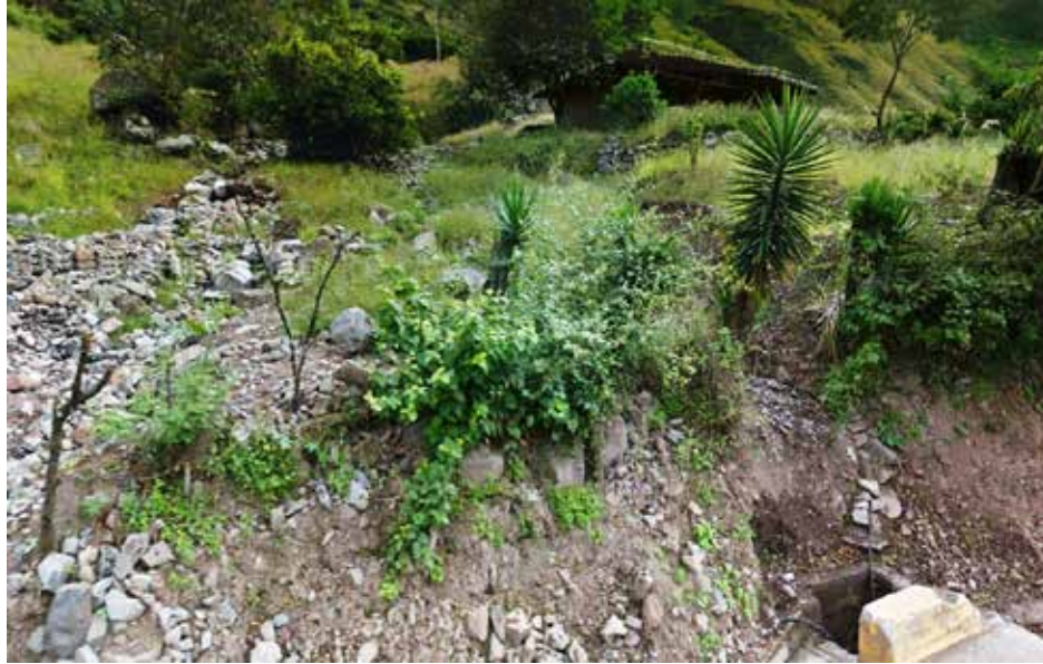
Photography 5.1.7: Colluvial deposit in k 0 + 600, clasts of andesitic lavas, volcanic scoria.
