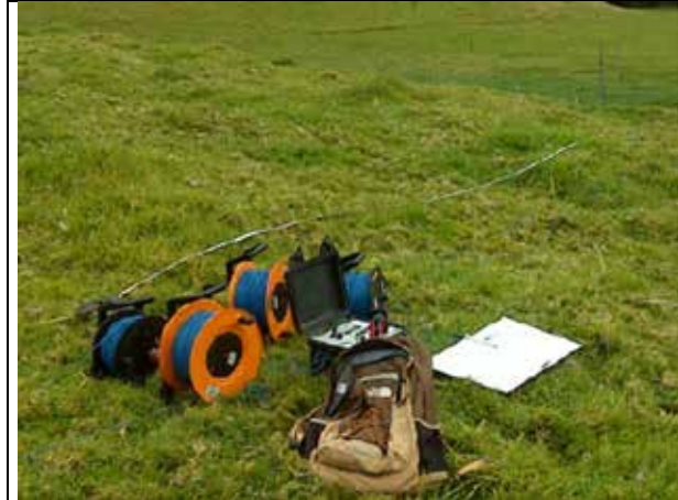
Photography 5.1.69 Allied Associates resistivity meter
