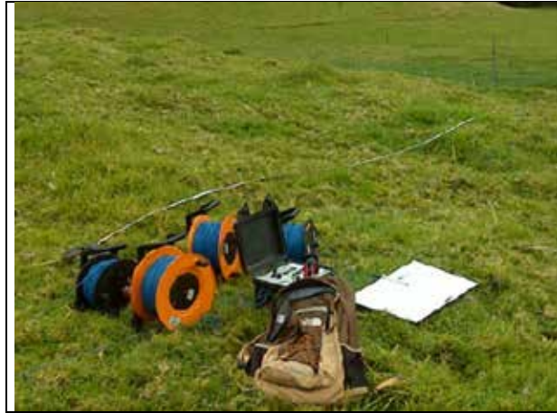
Photography 5.1.69 Allied Associates resistivity meter
