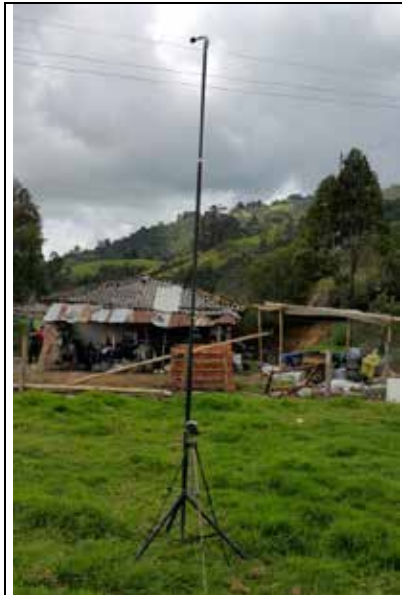
Photograph 5.1.79 Environmental noise measurement
