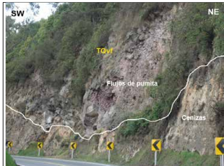
Photography5.1.10 Matrix pumice flows supported from unit TQvf, observed in the K30+300 Source (INGETEC, 2016)
