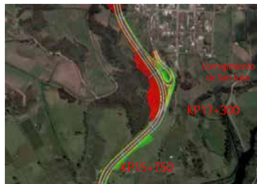
Photograph 3.14 KP17+000. Start point of the new divided highway to be built and interchange for access to the San Juan district - municipality of Ipiales. Coordinates E 947603 N 590068.
