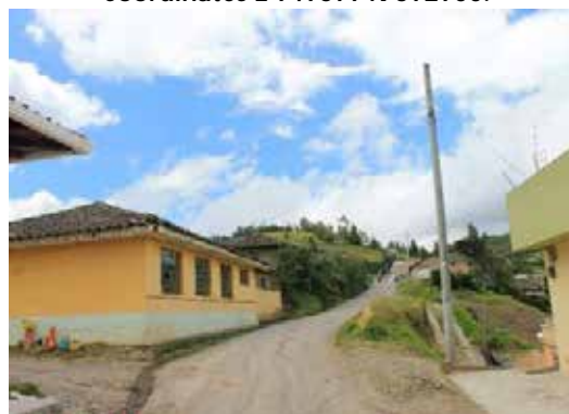
Photograph 3.31 KP3+358. Road section, granular material, roadway 4.50 m wide. Near to the populated area of the Aldea of María district - municipality of Contadero. Coordinates E 949699 N 592900.
