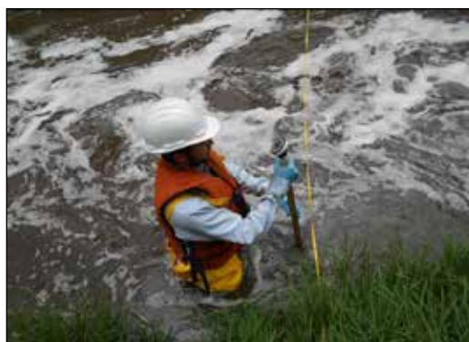
Picture 2.8 Flow Rate Measuring with a Propeller Flow Meter
