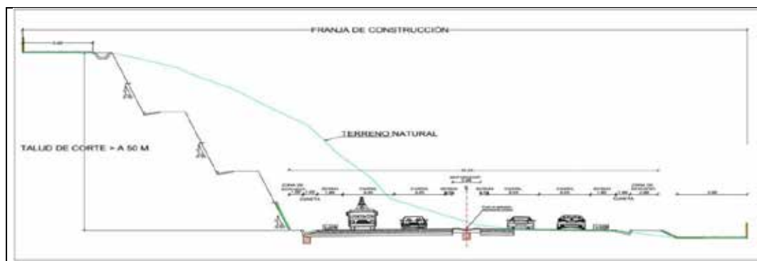
Figure 3.10 Proposed cross section for cut slopes greater than 50m
