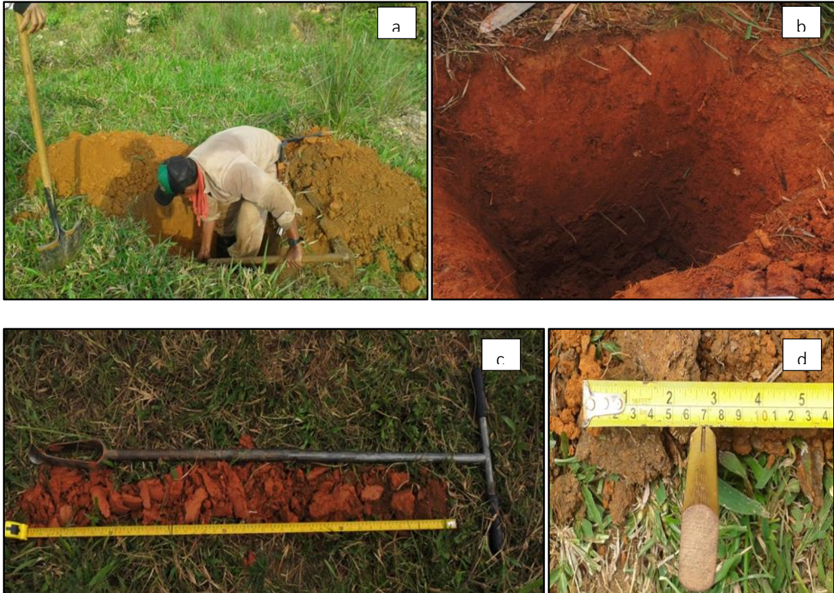
Illustration 1-14. a) Drilling taken in the project area b) Removal of soil with borehole. c and d. Measurement of horizons.
