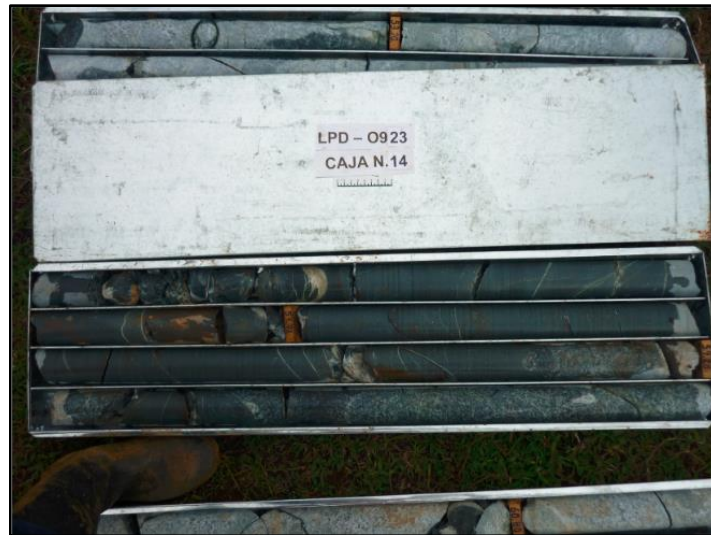
Illustration 2.2-18. Drilling cores ready for the logging process. Source: Touchstone Colombia, 2013
