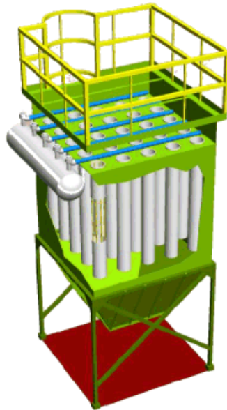
Illustration 8-24 Conceptual scheme of bag filter. Source: MAVDT 2010.
