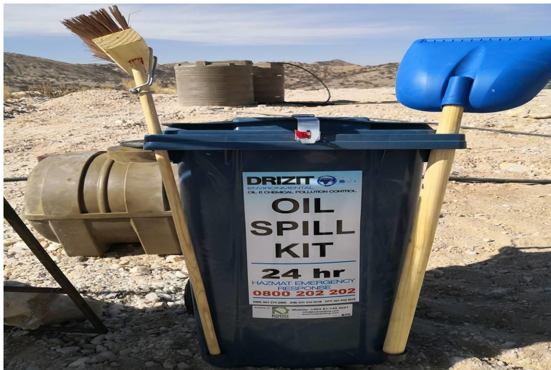
Figure 4 – Photo (DLE)- Oil spillage containment kit at one of the drill sites over a historical coarse mine dump
