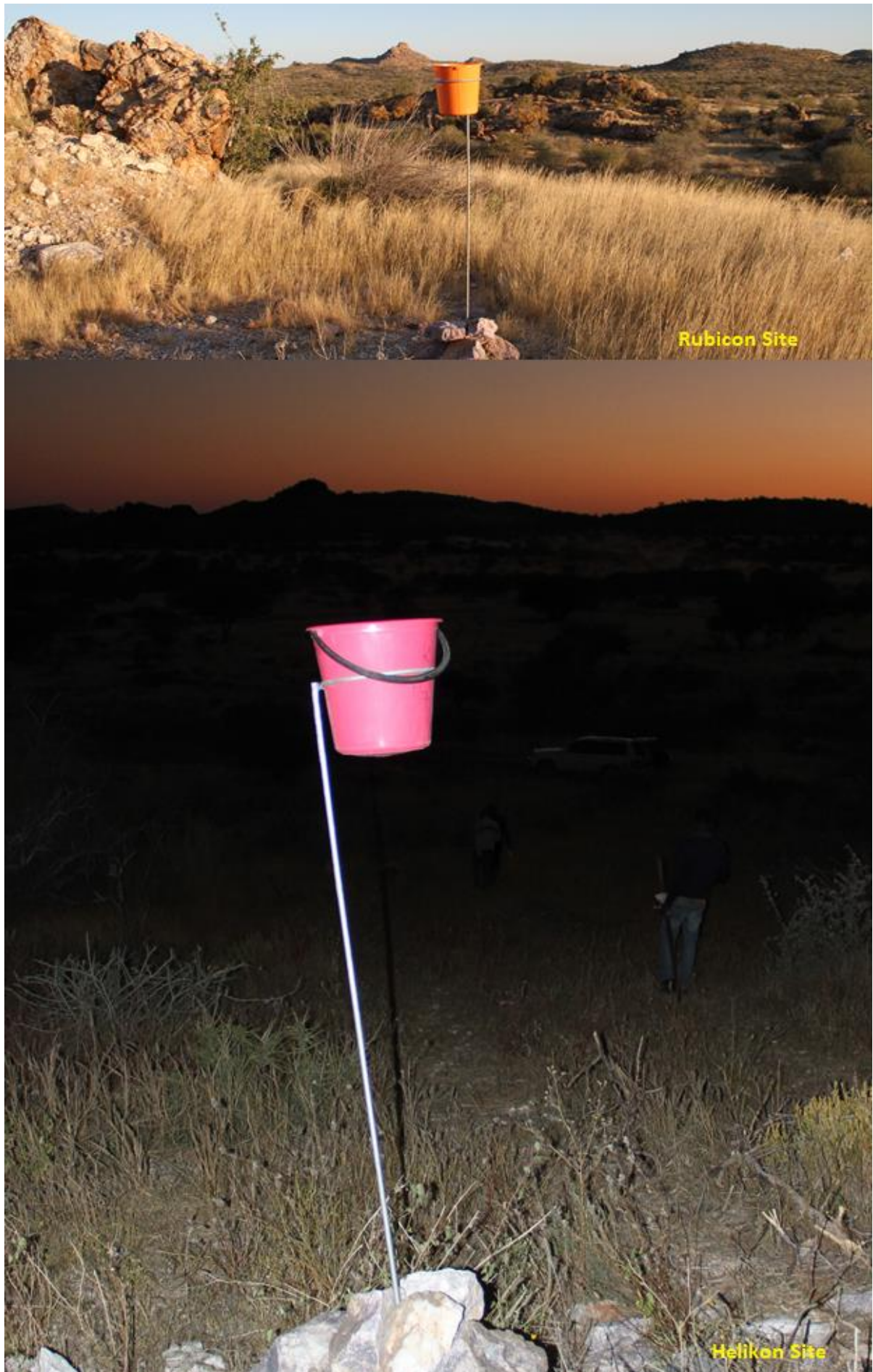
Plate 4.1: Rubicon and Helikon dust monitoring stations established within the ML 204 as part of the EIA process (RBS Geotagged Image Series, 2017).
