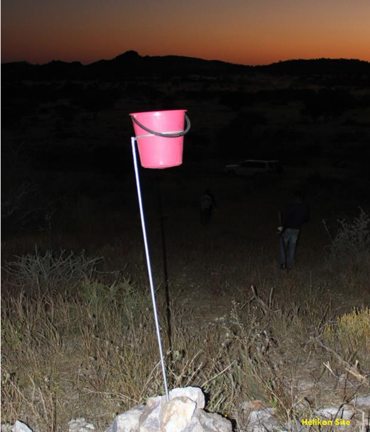
Plate 4.1: Rubicon and Helikon dust monitoring stations established within the ML 204 as part of the EIA process (RBS Geotagged Image Series, 2017).
