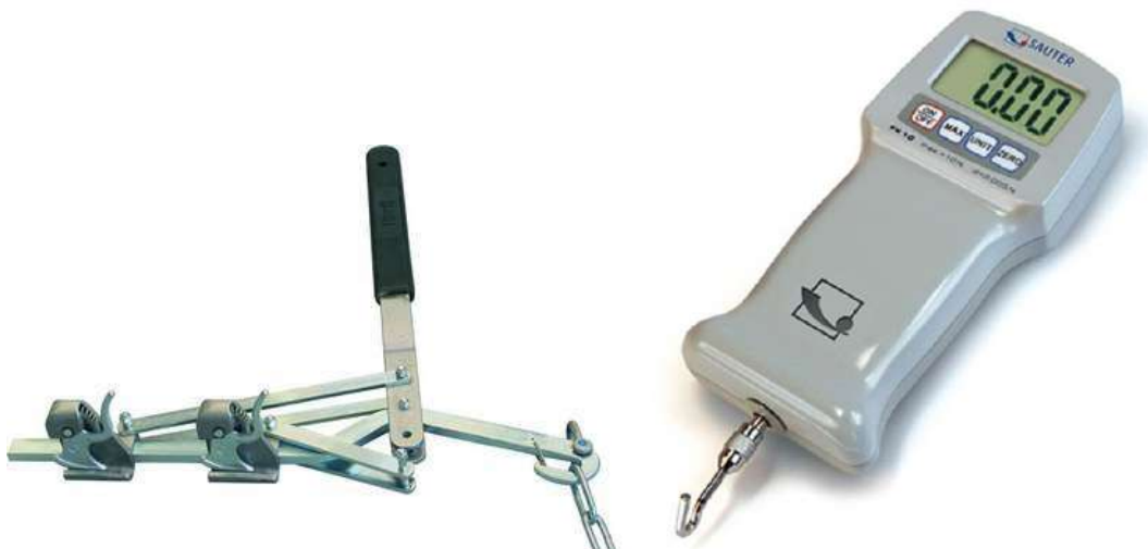
Illustration 9: Manual equipment of cable tension and cable tension meter. - Dynamometer
