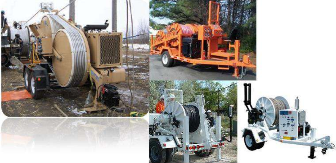
Illustration 4: VIEW OF TRACTION AND BRAKE EQUIPMENT USED IN LAYING AND TENSIONING ACTIVITY.
