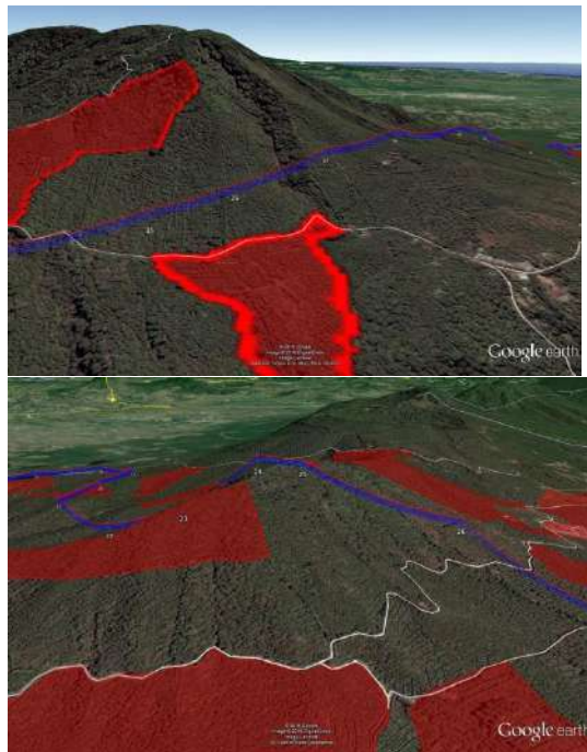
Figure 5.4-4 Transmission Line Avoiding Approach to Residential Zone in Ahuachapán The line has avoided passage through sensitive areas, as shown in Figure 5.4-5 below.
