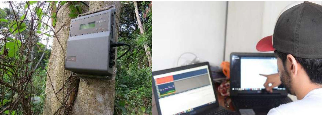
Figure 2. Installation of Acoustic Equipment SME3 and Analysis of Sonograms.
