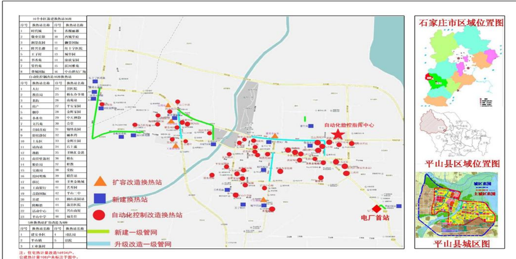
Figure 2 Location map of heating pipelines and heat exchange stations
