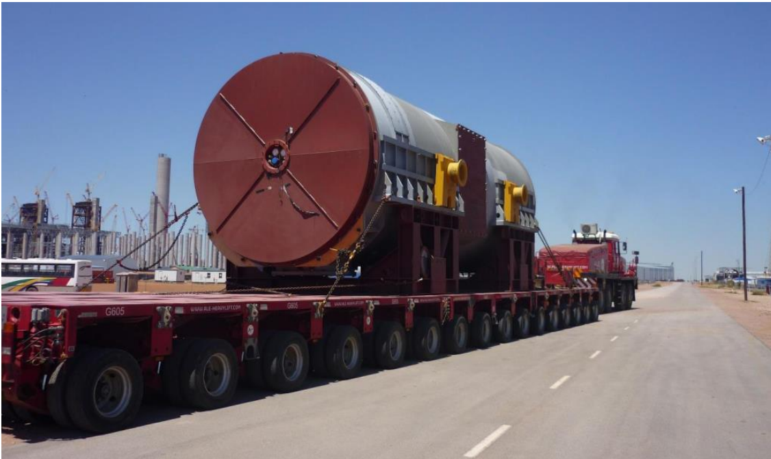
Figure 8: Heavy haulage truck with 16-axle hydraulic trailer transporting a 360 ton generator (source: ALE)
