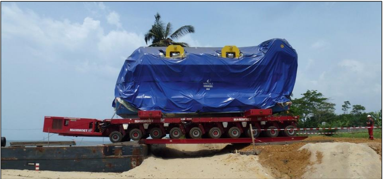
Figure 6: Example of trailer with load moving from temporary jetty onto land (source: SUBTECH)
