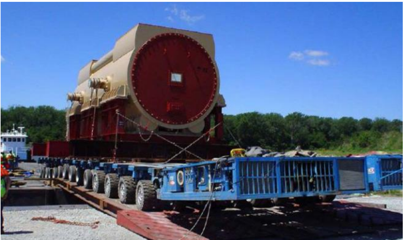
Figure 7: Example of large equipment being offloaded from a barge. Note the levels of the ramp, the barge and the jetty (source: SUBTECH)
