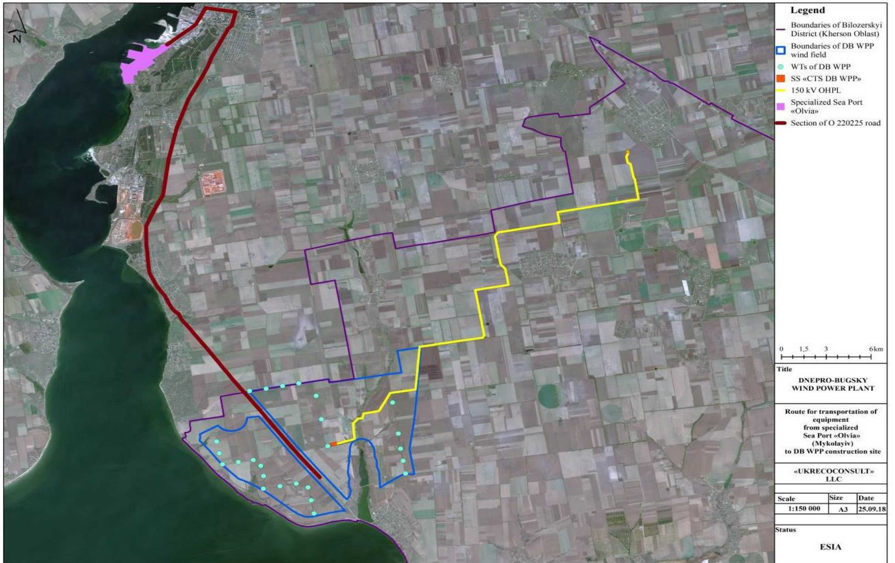
Fig. 8.3. Route for transportation of equipment from specialized Sea Port «Olvia» (Mykolayiv) to «DB WPP» construction site
