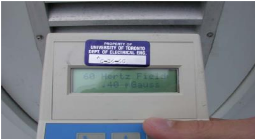
Fig. 4.97. The magnetic field measured in front of the steel door of the turbine tower with the magnitude of 0,4 mG
