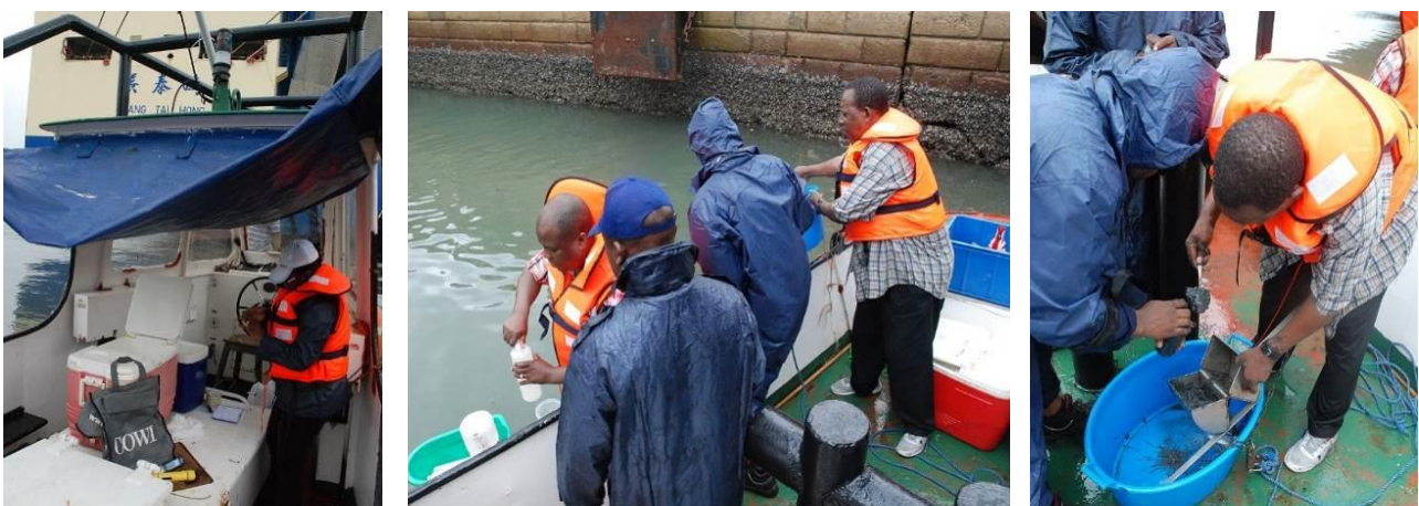
Figure 4-19 Recording position, depth data and water clarity data, and labelling sample containers (left), collection of water samples (centre) and extraction of sediment from Van Ven Grab (right), aboard the TPA Mooring Boat (15 December 2015).
