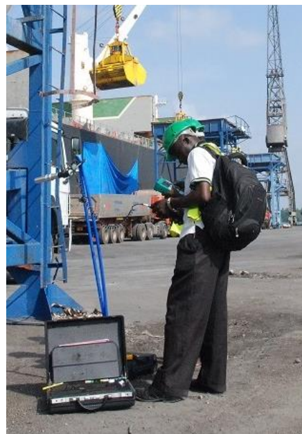
Figure 4-21 Recording noise, air quality and vibrations, during fertiliser unloading via hoppers into trucks. January 2016.
