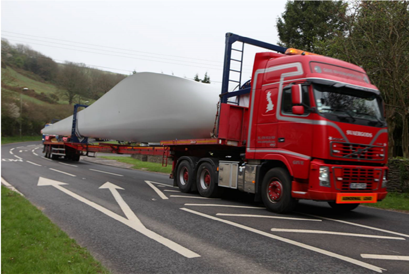
Figure 14-4: Turbine Blade in transportation
