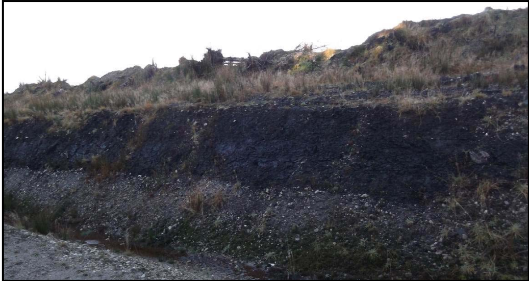
Plate 17-40: Exposed edge showing peat overlying gravelly subsoil
