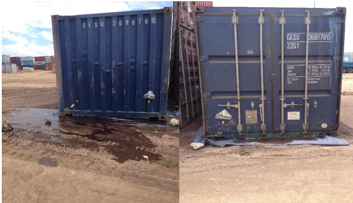
Fig. 5-2: Observed chemical leakage from containers and its out-dated management
