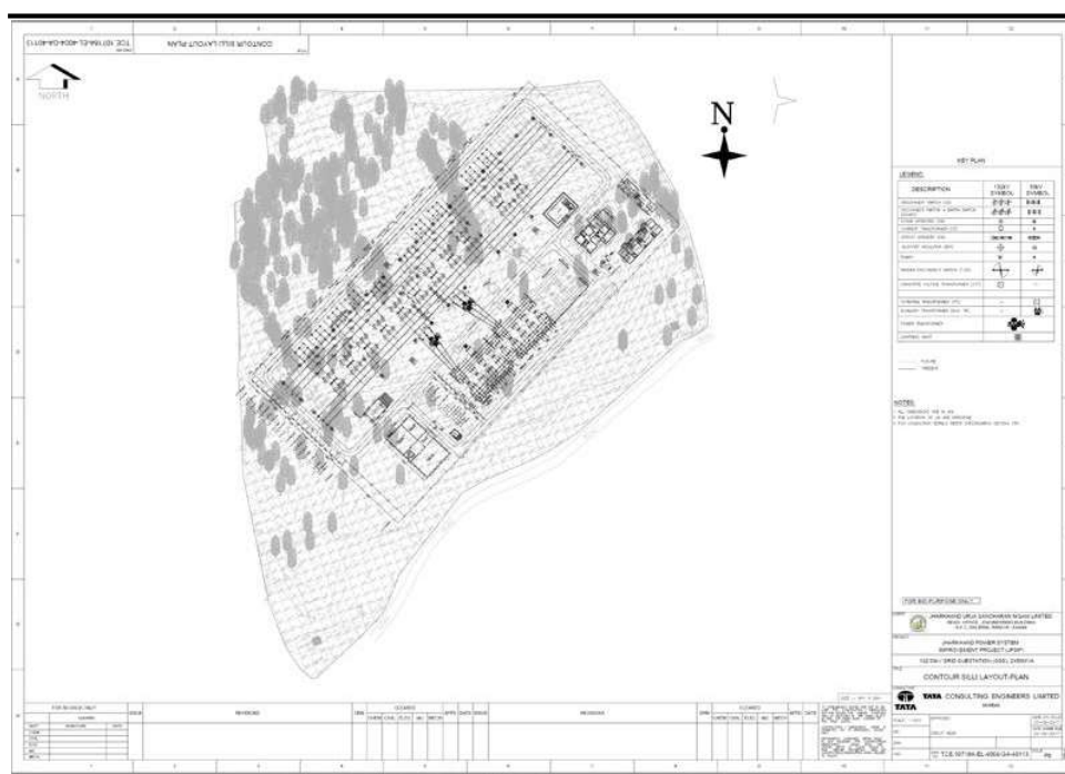
Figure 3.4 Layout of a 132/33 KV substation at Silli Planned in the JPSIP
