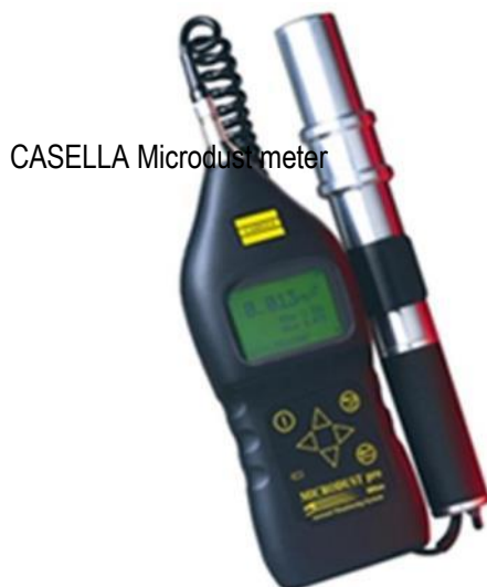
Photo 3: Digital CASELLA microdust and 6-gas MX6 iBrid™ meters to be used to measure air quality
