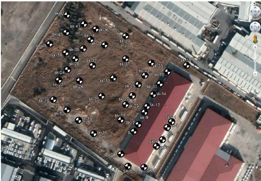
Figure 6-3: Locations of the boreholes drilled during the ground survey study
