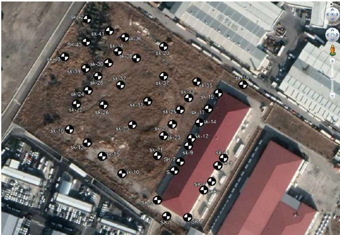
Figure 6-3. Drilling and sampling were performed according to TS 1901-1 and TS EN ISO 22475-1 standards. Studies were carried out using hydraulic drilling machinery and equipment.
