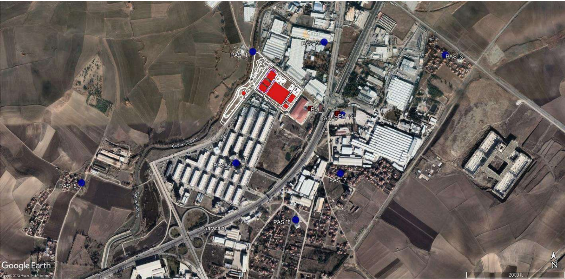
Figure 9-4: Baseline Ambient Air Quality Measurement Locations (PM_x: Particulate matter and dust deposition monitoring locations, PAS_x: Passive gas sampling locations)
