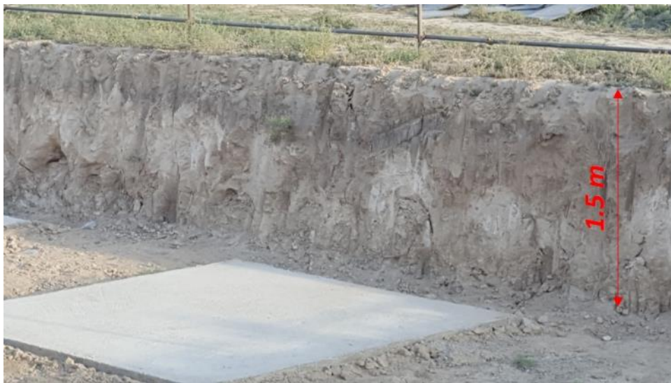
Figure 7.6.2: Profile of a typical (Haplic) Calcisols of the Project Area
