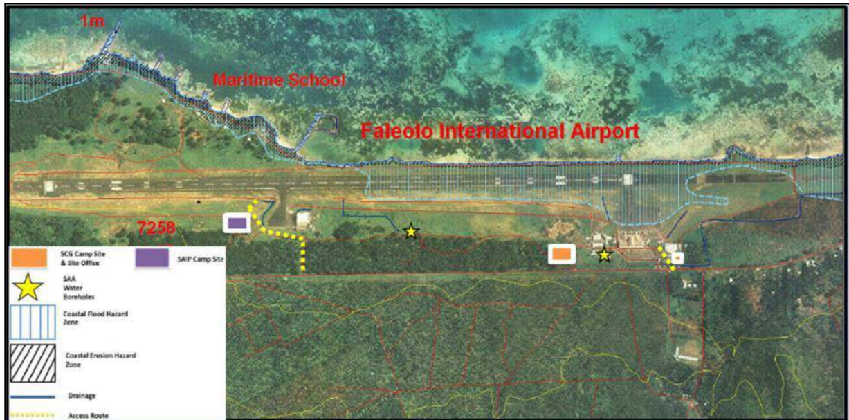
Figure 11: The potential coastal flood hazard at the Faleolo International Airport (APW) (Source: CB Group, 2015 via AECOM SAIP IESMP.)
