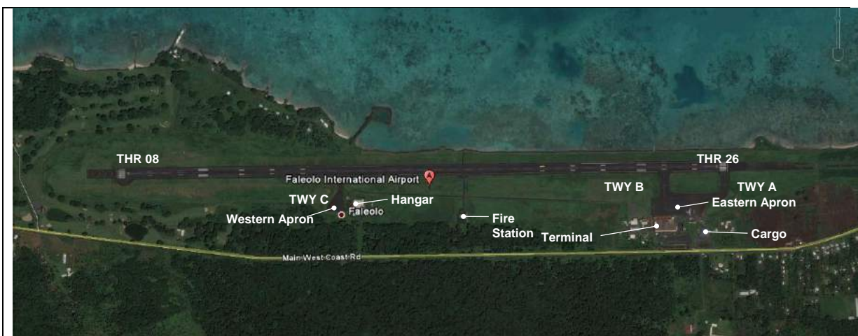
Figure 3: APW general existing airport layout (Source: Aerial photography from Google Earth Pro, dated 4 January 2015 via AECOM SAIP IESMP.)
