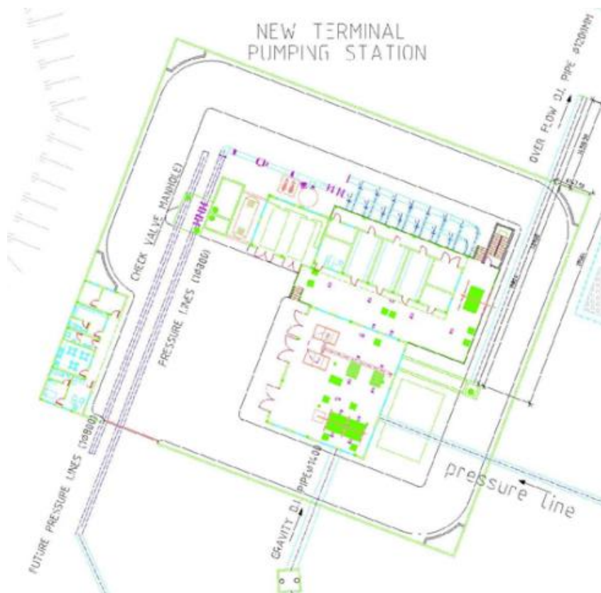
Figure 3.1 General Layout of the terminal pumping station (TPS).
