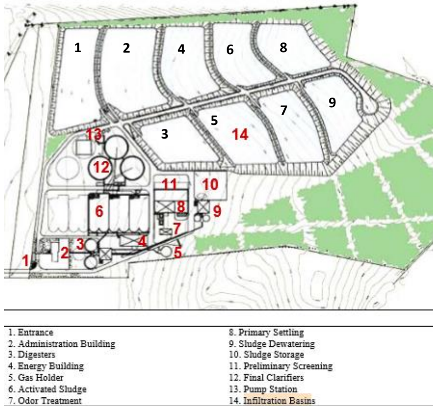
Figure 3.2 General Layout of the NGWWTP
