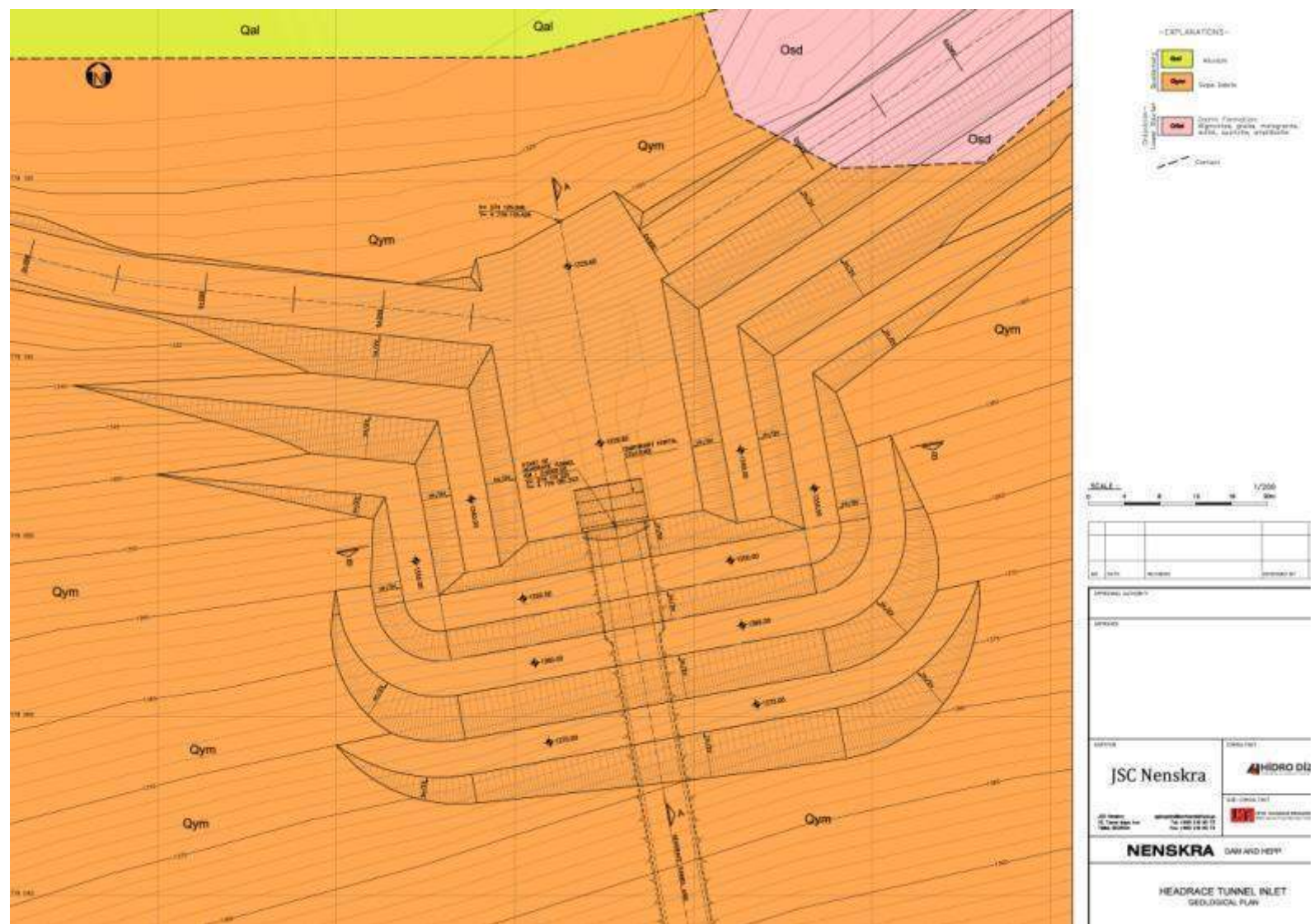
Figure 5.2.3.6.2.3.6. Entrance of headrace tunnel (geological plan)
