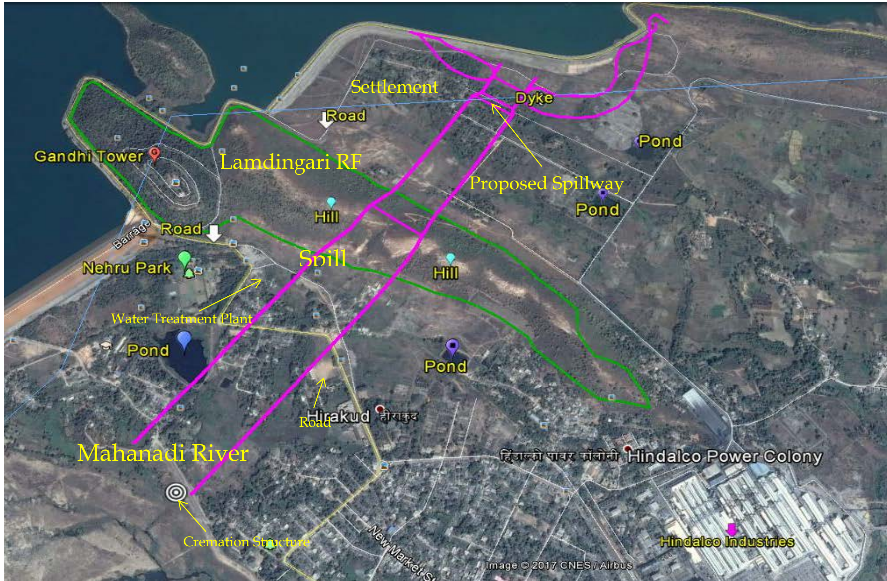
Fig. 3-6: Environmental features in and around the proposed Additional Spillway
