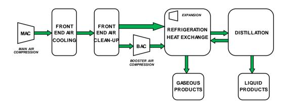
Air Separation is a physical process that produces oxygen, nitrogen and argon by cryogenic (low temperature) distillation of air. The only substantial inputs are air from the atmosphere and electricity; the only emissions from the process itself are air gases returned to the atmosphere.
