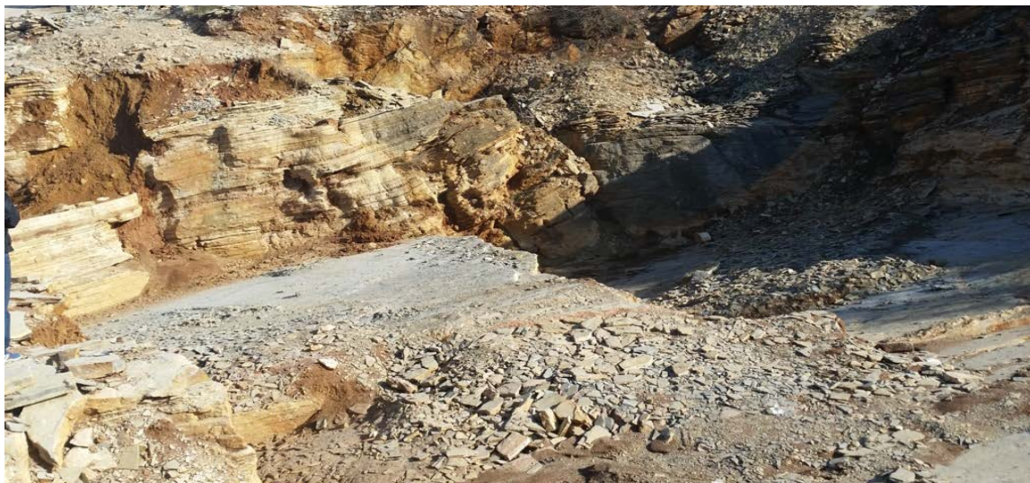
Figure 30: Km cca 6+000: Flysch sediments consisting of marl, sandstone, marly limestone and massive to blocky limestone appropriate for embankment
