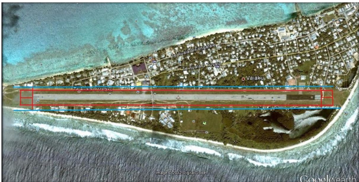
Figure 1: Funafuti Airport with the existing 80m runway strip and transitional OLS protection limit for structures of 4m shown as blue line.
