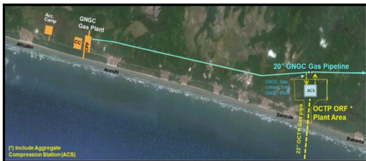
Figure 3: OCTP Non-associated Gas Development – Onshore Receiving Facility
