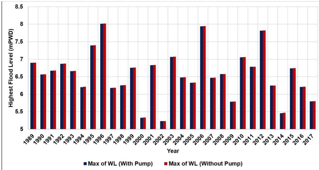
Figure 7.5: Highest Flood Level With and Without Pump
