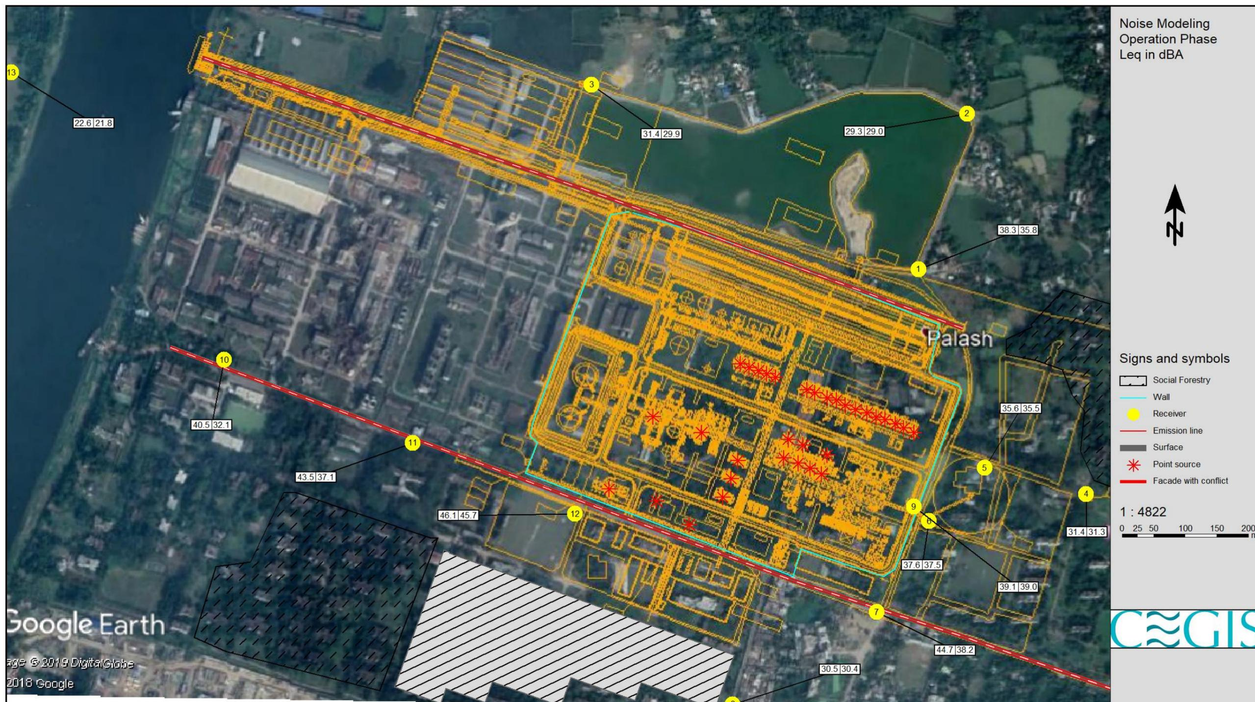
Figure 7.9: Noise level at different sensitive receptors during Plant Operation
