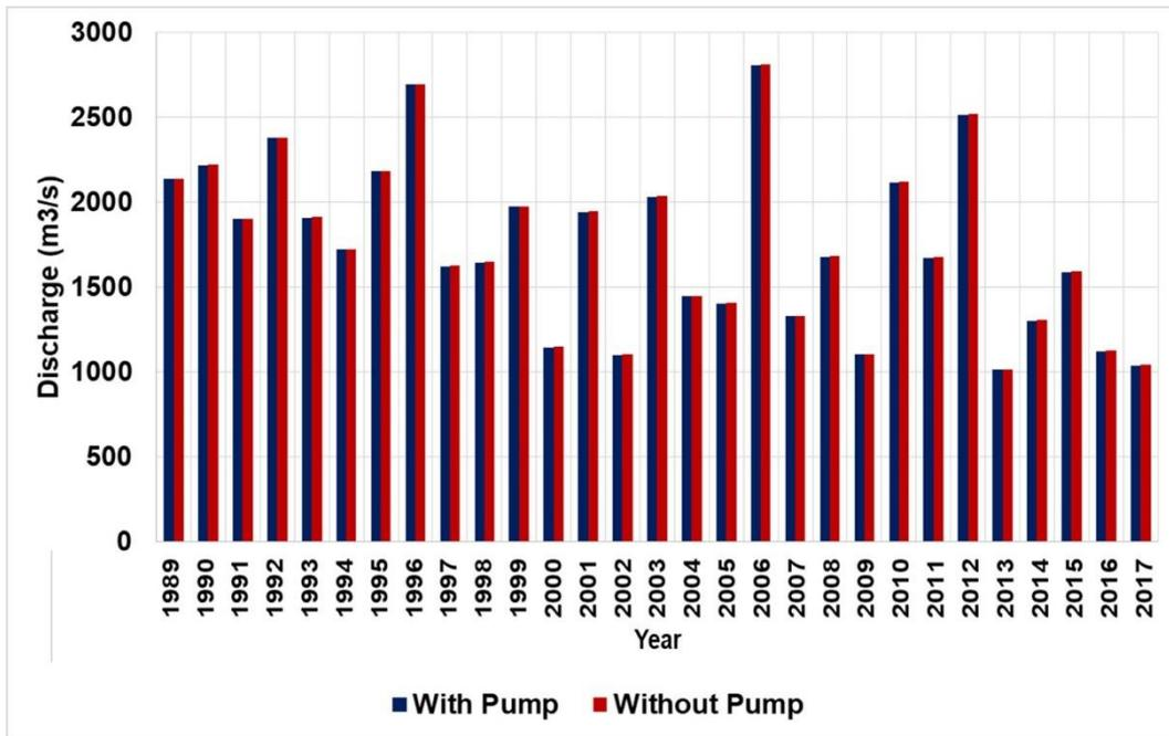
Figure 7.7: High Discharge Rate With and Without Pump
