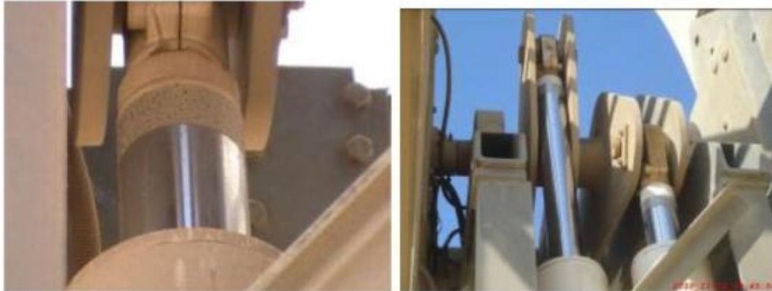
Figure 9: Pitting Occurred on the Chromatic Surface of the Drive Pylon Piston
