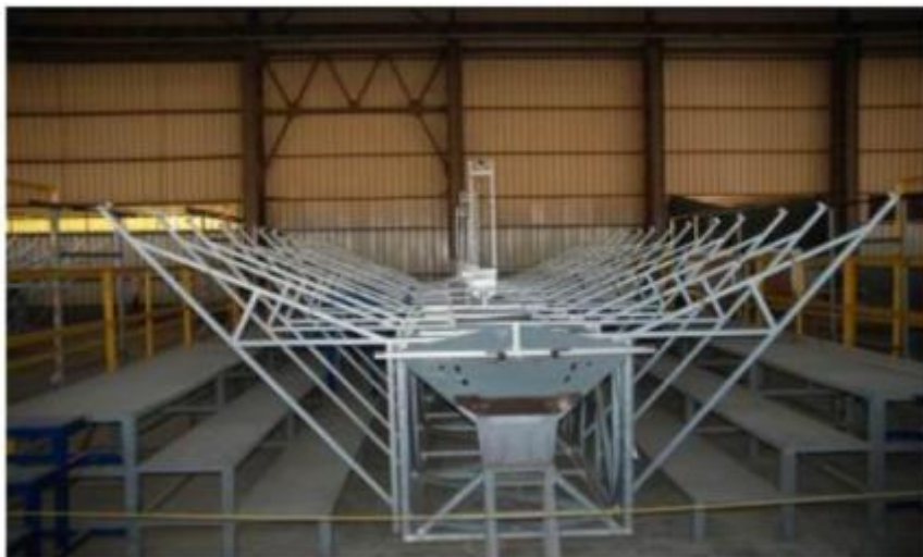
Figure 7: Photogrammetry Station to Assure the Quality of the Assembly
