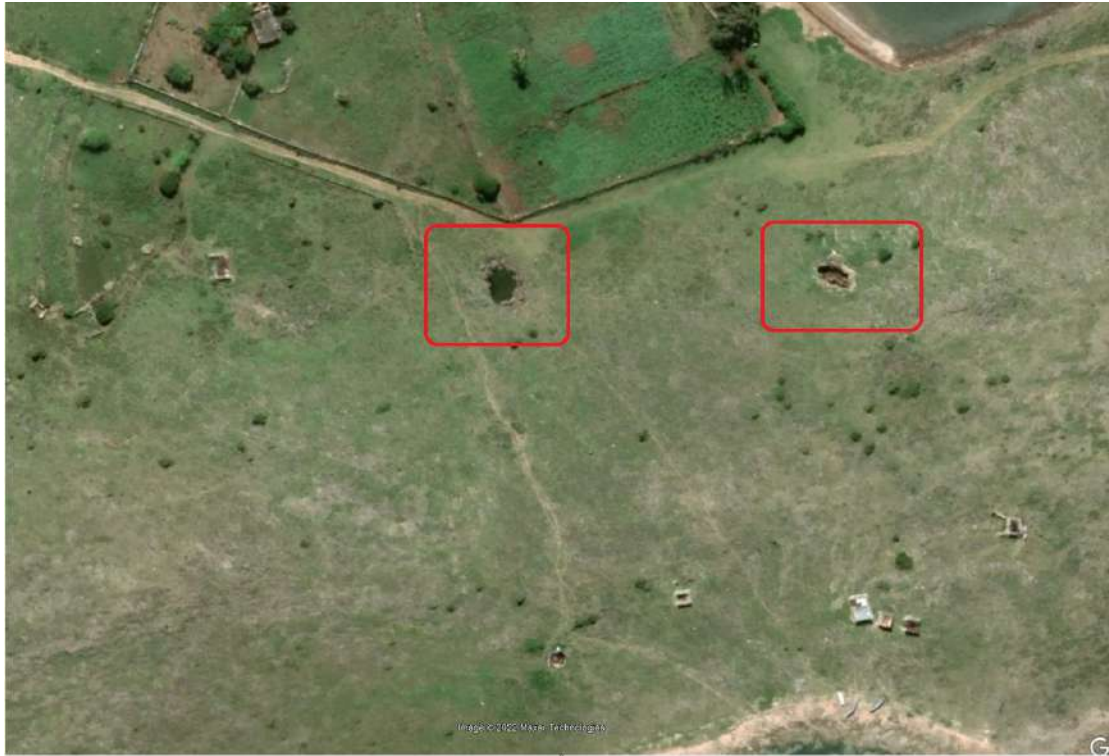
Figure 2: Positions of ground features in the South East of the Site associated with Karstic Ground Conditions
