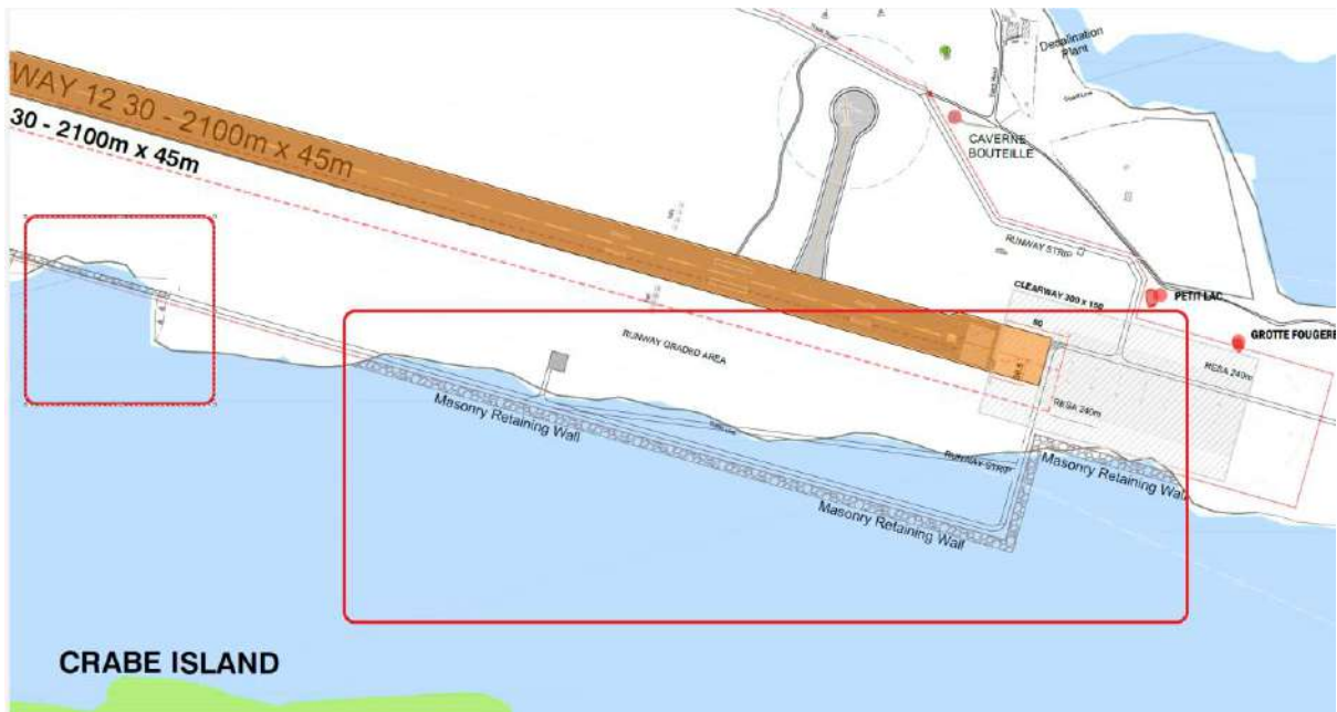
Figure 3: Blow up of Proposed Runway showing extent to be built offshore. Note Positions of ground features such as Petit Lac, Grotte Fougere and Cavern Bouteille
