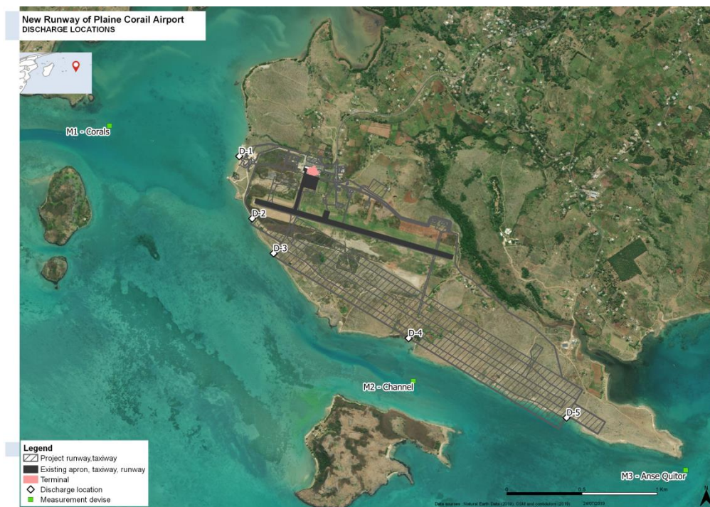
Figure 171: Localization of the potential sediment discharges to the lagoon during works phase and current-meter
