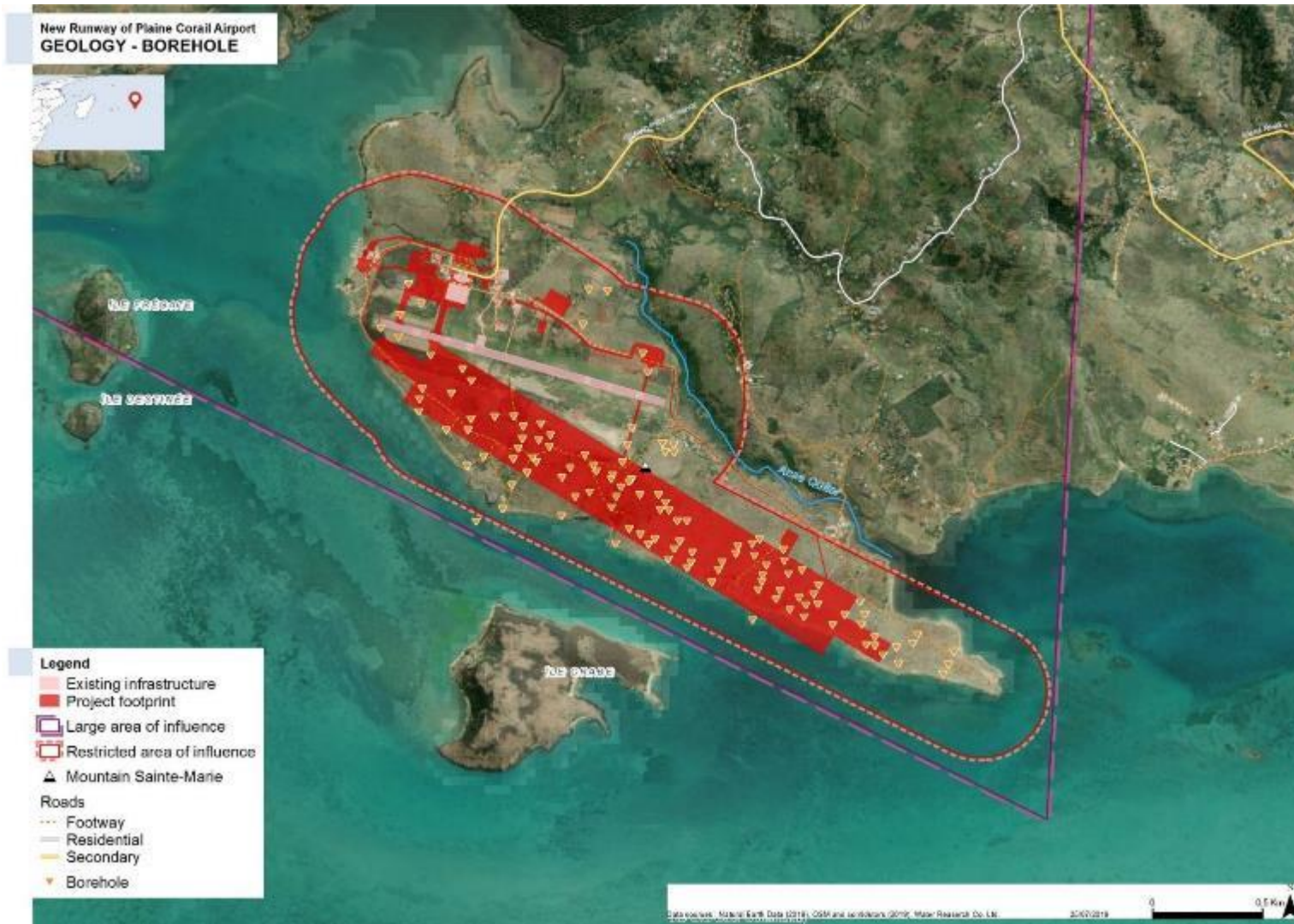
Figure 2-11: All ground investigations from Phase B (2017) and Phase C (2018) geotechnical campaign of the restricted area of influence at Plaine Corail (Preliminary Design, 2017) – Boreholes
