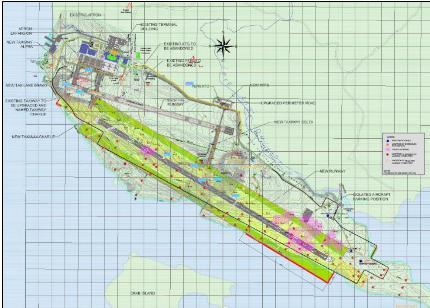
Figure 2-12: All ground investigations from Phase B (2017) and Phase C (2018) geotechnical campaign of the restricted area of influence at Plaine Corail (Preliminary Design, 2017)
