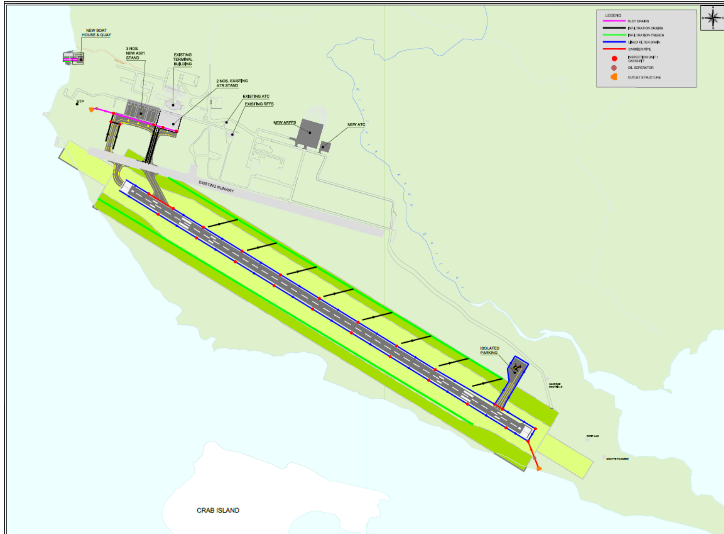
Figure 1-13: Surface Water Drainage: Drawing No. M243/DD/CE/SK/16
