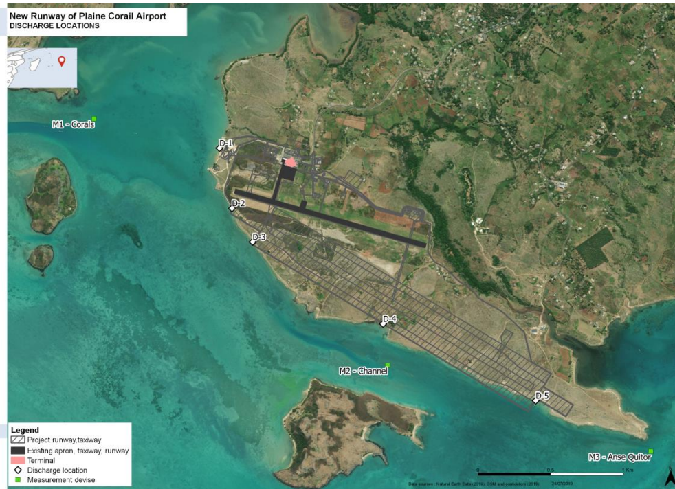
Figure 29 Localization of the potential sediment discharges to the lagoon during works phase and current-meter
