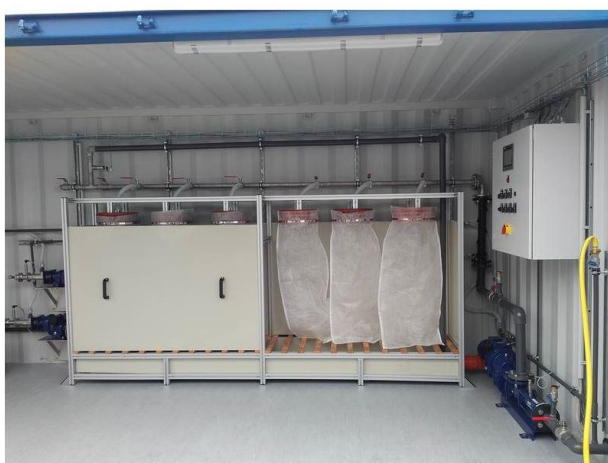
Figure 4: Example of the filtration bag technology proposed for the sludge treatment on site
