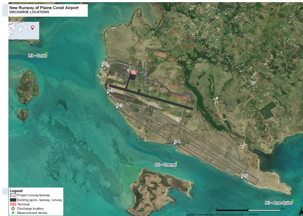
Figure 22: Localization of the potential sediment discharges to the lagoon during works phase and current-meter
